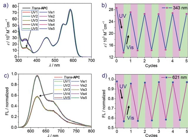
**Fig. 4** Absorption and emission spectrum switching under alternate UV (350 nm) and visible light irradiation. (a) UV-vis absorption spectra of cyclophane APC ( $[APC] = 8.6 \times 10^{-6}$  M in DCM). (b) Change of azobenzene absorption at 343 nm. (c) Fluorescence spectra of APC. (d) The emission intensity changes at 621 nm. The UV irradiation time is 60 s for each cycle and the visible light irradiation time is 10 min.
