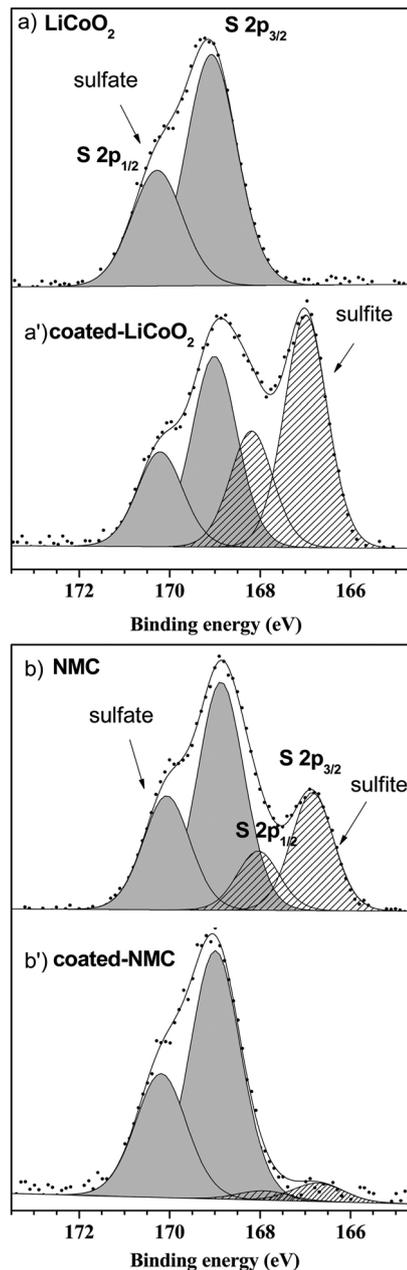
Fig. 5 XPS spectra for the S 2p core peaks after  $\text{SO}_2$  adsorption on (a)  $\text{LiCoO}_2$  and (a')  $\text{Al}_2\text{O}_3$  coated  $\text{LiCoO}_2$  and XPS spectra for the S 2p core peaks after  $\text{SO}_2$  adsorption on (b) NMC and (b')  $\text{Al}_2\text{O}_3$  coated NMC. Reprinted (adapted) with permission from ref. 104. Copyright (2015) American Chemical Society.
