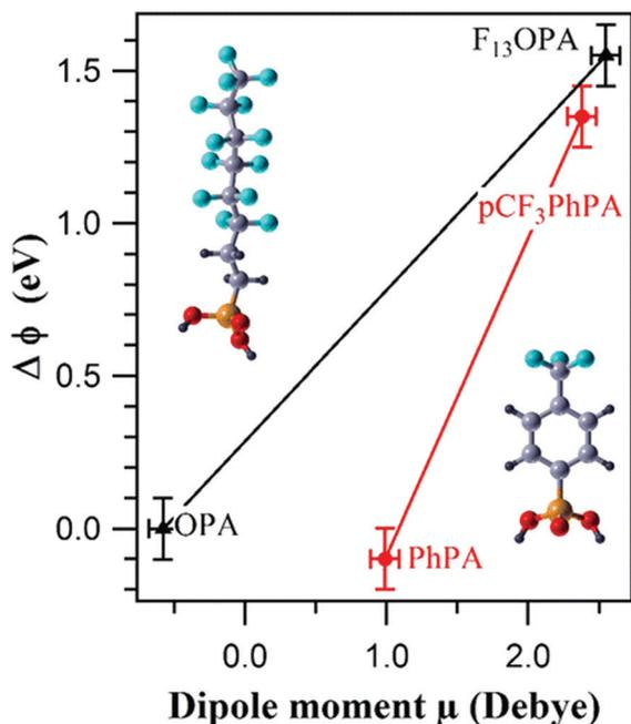
Fig. 15 Correlation between the experimental change in work function ( $\Delta\phi$ ) and the molecular dipole moment  $\mu$  of the PA molecules for 3,3,4,4,5,5,6,6,7,7,8,8,8-tridecafluorooctyl phosphonic acid-(( $\text{F}_{13}$ )OPA, left molecule in figure) and *p*-(trifluoromethyl)phenylphosphonic acid-(( $\text{pCF}_3$ )PhPA, right molecule in figure) modified ZnO surfaces, along with corresponding non-fluorinated analogues.<sup>273</sup>
