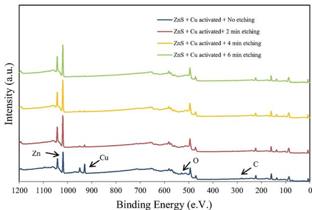
Fig. 9 Survey spectra of copper activated sphalerite after; no etching, 2 minutes, 4 minutes, and 6 minutes of etching corresponding to a depth of 3, 6, 10 nm respectively Reprinted from Ejtemaei *et al.*, Characterisation of sphalerite and pyrite surfaces activated by copper sulfate, *Miner. Eng.*, 2017, **100**, 223–232, Copyright (2007), with permission from Elsevier.<sup>148</sup>
