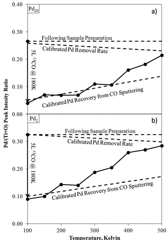
Fig. 12 Pd/(Ti + O) ISS intensity ratios for Pd<sub>20</sub>/TiO<sub>2</sub> (a) and Pd<sub>2</sub>/TiO<sub>2</sub> (b) as-deposited, after exposure to CO at 180 K, and during temperature ramping. Calibrated rates for recovery of Pd from ISS sputtering.<sup>171</sup> Calibration lines account for unintended sputtering effects from the ISS experimental conditions selected for this analysis. Deviations from this calibration indicate a changing surface structure (desorption of CO).
