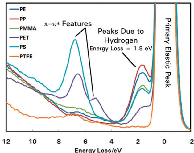
Fig. 18 REELS spectra of polyethylene, polypropylene, poly(methyl methacrylate), polyethylene terephthalate, polystyrene and poly tetrafluoroethylene to evidence the changing peak intensity at  $\sim 1.8$  eV with differing H concentration. Reprinted (adapted) with permission from ref. 391. Copyright (2013) Thermo Scientific.
