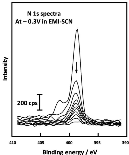
Fig. 6 XPS depth profiling spectra of the N 1s level from Mn oxide electrodes in EMI-SCN, [C<sub>2</sub>C<sub>1</sub>Im][SCN] polarised at  $-0.3$  V, reported by Chang *et al.* Reprinted (adapted) with permission from ref. 122. Copyright (2009) American Chemical Society.
