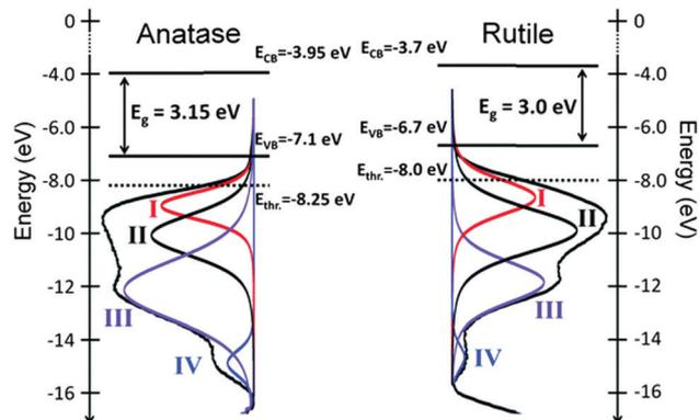
Fig. 14 He(I) UPS profiles, fit with an established empirical model and an overlaid electronic structure of the two  $\text{TiO}_2$  polymorphs anatase and rutile relative to the vacuum level.  $E_{\text{thr}}$  corresponds to the deepest state that can be excited in a photocatalytic test ( $E_{\text{photons}} \leq 4.3$  eV).<sup>262</sup>
