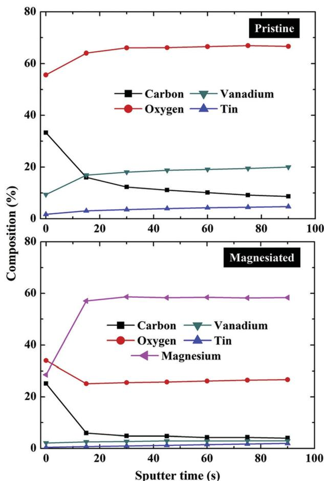
Fig. 3 XPS depth profile composition measurements of pristine and magnesiated V<sub>2</sub>O<sub>5</sub> cathodes indicating the relative contents of carbon, oxygen, vanadium, tin and magnesium as a function of overall ion bombardment time (in itself a function of depth from the surface of the sample down into the bulk).<sup>89</sup>
