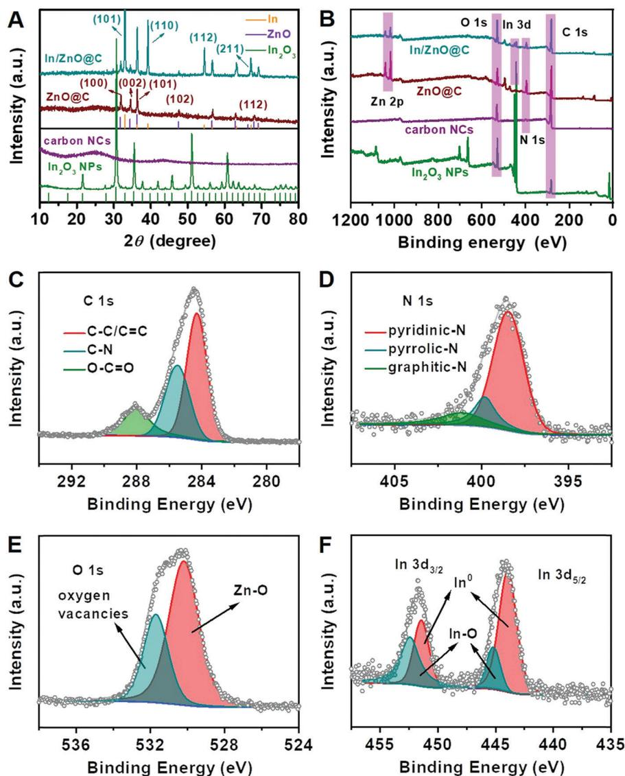
Fig. 2 (A) XRD patterns and (B) full XPS spectra of In/ZnO@C, ZnO@C, carbon NCs, and In<sub>2</sub>O<sub>3</sub> NPs. High-resolution XPS spectra of (C) C 1s, (D) N 1s, (E) O 1s and (F) In 3d for In/ZnO@C.
