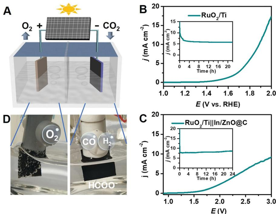
Fig. 4 (A) Schematic illustration of the CO<sub>2</sub>RR-OER full cell. (B) OER polarization curve and electrolysis curve at 1.8 V for RuO<sub>2</sub>/Ti in 0.5 M KHCO<sub>3</sub>. (C) CO<sub>2</sub>RR-OER polarization curve and electrolysis curve with an applied cell voltage of 2.7 V for the full cell. (D) Digital images showing the bubbles on two electrodes during solar-driven CO<sub>2</sub>RR-OER electrolysis.
