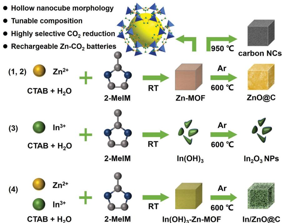
Scheme 1 Schematic illustration of the fabrication of carbon NCs, ZnO@C NCs, In<sub>2</sub>O<sub>3</sub> NPs and In/ZnO@C NCs as CO<sub>2</sub>RR electrocatalysts.
