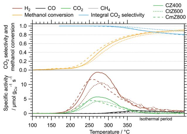
**Fig. 3** MSR profiles of CZ400, CtZ600 and CmZ800 between 100 °C and 350 °C including an isothermal period of 30 min. Colour code: orange – methanol conversion, blue – integral CO<sub>2</sub> selectivity, specific activity of brown: H<sub>2</sub>, black: CO, green: CO<sub>2</sub>, grey: CH<sub>4</sub>. Heating rate: 5 °C min<sup>-1</sup>; sample mass: CZ400 – 18.6 mg, CtZ600 – 21.6 mg, CmZ800 – 20.2 mg.
