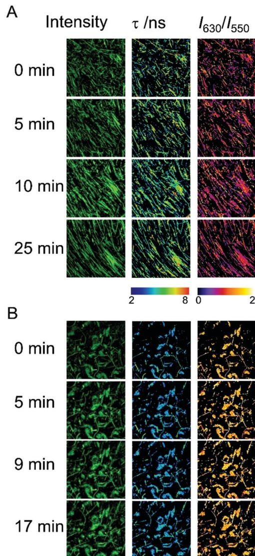
Fig. 6 Intensity, FLIM, and ratiometric images of the dye **AQui** in self-healing Fmoc-FF hydrogels formed with Ca<sup>2+</sup> (A) and Cs<sup>+</sup> (B) after ultrasound treatment, as a function of time. The size of the images is 10  $\mu\text{m} \times 10 \mu\text{m}$ .
