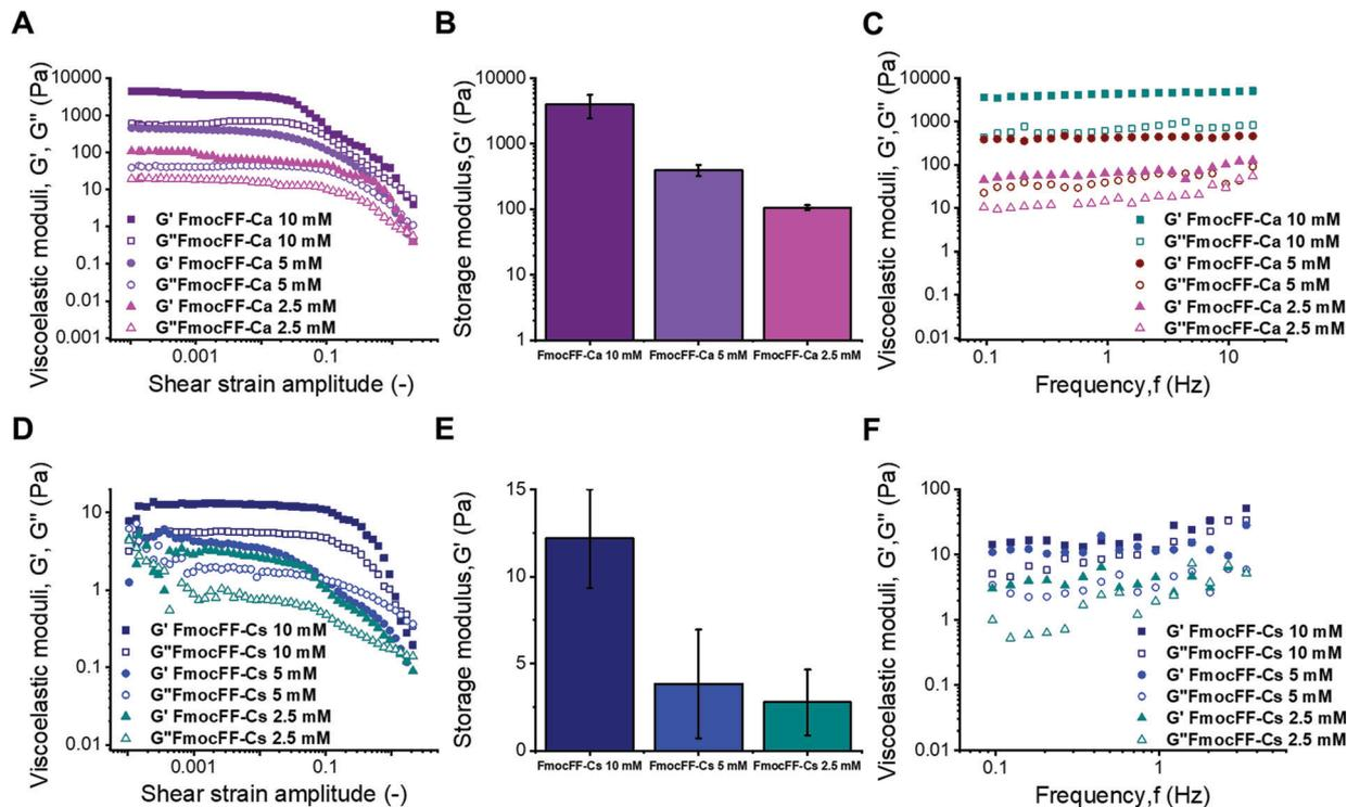
Fig. 5 Mechanical characterization of the samples under oscillatory shear. (A) and (C) show the amplitude and frequency sweeps for  $\text{Ca}^{2+}$  samples, and (B) the mean and standard deviation of the storage modulus corresponding to the linear viscoelastic region. (D)–(F) show the same results but for  $\text{Cs}^{+}$  samples.
