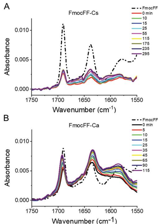
Fig. 3 Time-dependent FTIR spectra of Fmoc-FF Cs<sup>+</sup> (A) and Fmoc-FF Ca<sup>2+</sup> (B) salt hydrogels (10 mM peptide conc.).
