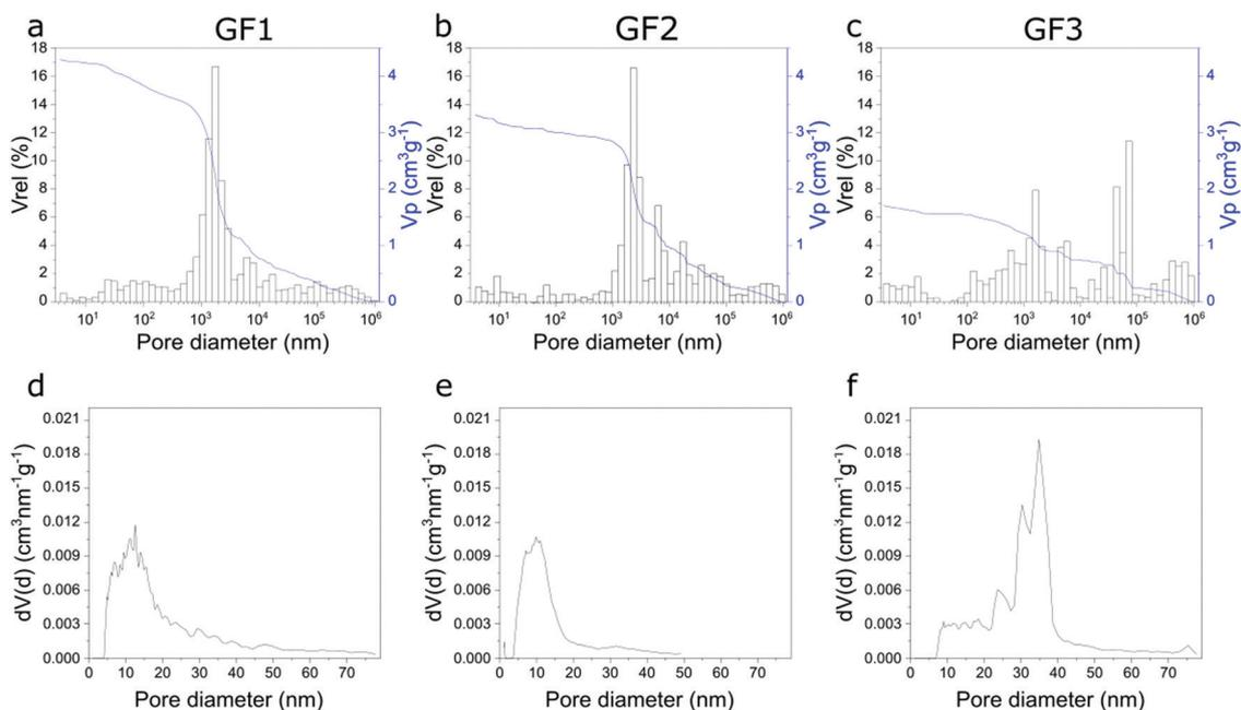
Fig. 3 Pore width distributions of samples GF1, GF2 and GF3 obtained using Hg intrusion (a–c), and N<sub>2</sub> sorption (d–f).
