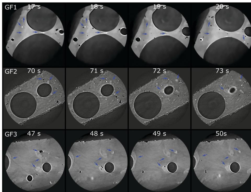
**Fig. 8** Micro-CT micrograms of samples GF1 (top), GF2 (middle), and GF3 (bottom) corresponding to frames of the Movies S1–S3 (ESI†), which show virtual slices of each sample when moving orthogonally to the sample's center of rotation. Blue arrows indicate some regions with bright spots attributed to manganese oxide residues occurring in the GF walls.
