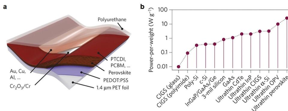
Fig. 4 Power-per-weight analysis. (a) Schematic diagram of the ultrathin perovskite solar cell. (b) Power-per-weight of various photovoltaic technologies. Reproduced with permission.<sup>7</sup> Copyright 2015, Springer Nature.
