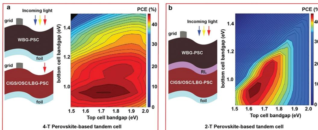
**Fig. 3** Structure and simulated efficiency of flexible tandem solar cells. (a) 4-T tandems and (b) 2-T tandems. Reproduced with permission.<sup>43</sup> Copyright 2020, Wiley-VCH.
