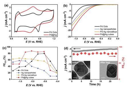
Fig. 6 CO<sub>2</sub>RR performance in CO<sub>2</sub>-saturated 0.5 M KHCO<sub>3</sub>. (a) CV curves without bubbling CO<sub>2</sub>; (b) polarization curves; (c) FE of CO at various applied potentials; (d) long-term i-t curve and CO FE, along with TEM images before and after electrolysis (scale bar: 20 nm).
