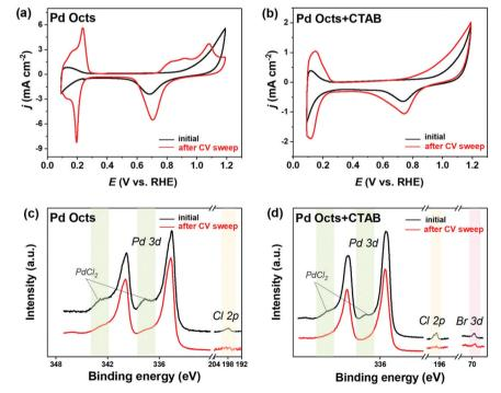
Fig. 4 Comparison of electrochemical surface cleaning for Pd Octs and Pd Octs with CTAB in 0.5 M H<sub>2</sub>SO<sub>4</sub>. (a and b) CVs and (c and d) XPS profiles of (a and c) Pd Octs and (b and d) Pd Octs with CTAB, before and after surface cleaning by CV sweeping
