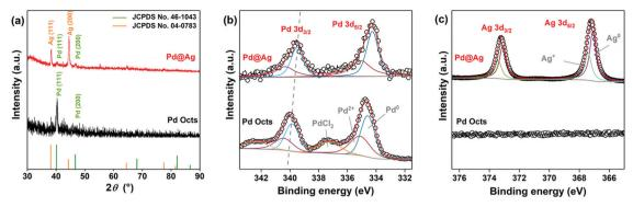
Fig. 2 (a) XRD patterns and XPS profiles of (b) Pd 3d and (c) Ag 3d of Pd@Ag cubes and Pd Octs.
