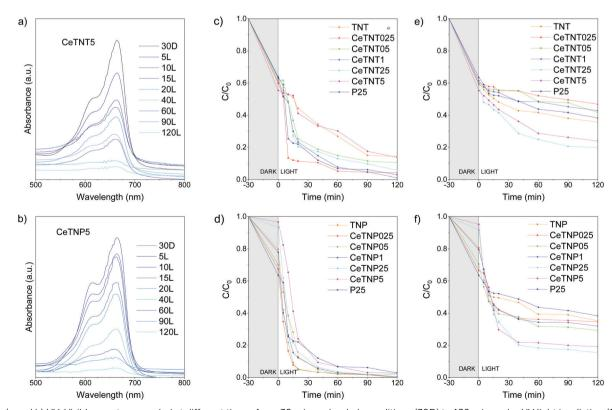
Fig. 4 (a and b) UV-Visible spectra recorded at different times, from 30 min under dark conditions (30D) to 120 min under UV light irradiation (120L), for the two 5.0 wt% CeO<sub>2</sub>-TiO<sub>2</sub> nanostructures: (a) CeTNT5 sample and (b) CeTNP5 sample. (c-f) MB photodegradation test in aqueous solution: CeTNTx (c) under UV light irradiation and (e) under simulated solar light; and CeTNPx (d) under UV light irradiation and (f) under simulated solar light.
