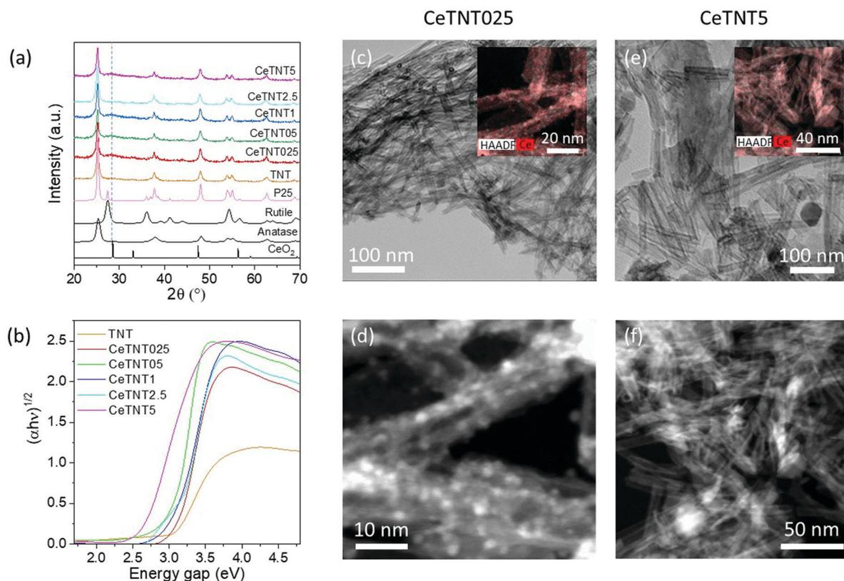
Fig. 1 Undoped and Ce-doped TNT series. (a) XRD patterns, including benchmarking anatase, rutile and P25. (b)  $(\alpha h\nu)^{1/2}$  vs. photoenergy (eV) plot. TEM/HAADF images for samples CeTNT0.25 (c and d) and CeTNT5 (e and f). The insets in (c) and (e) show the EDS maps for Ce overlapping the STEM images.
