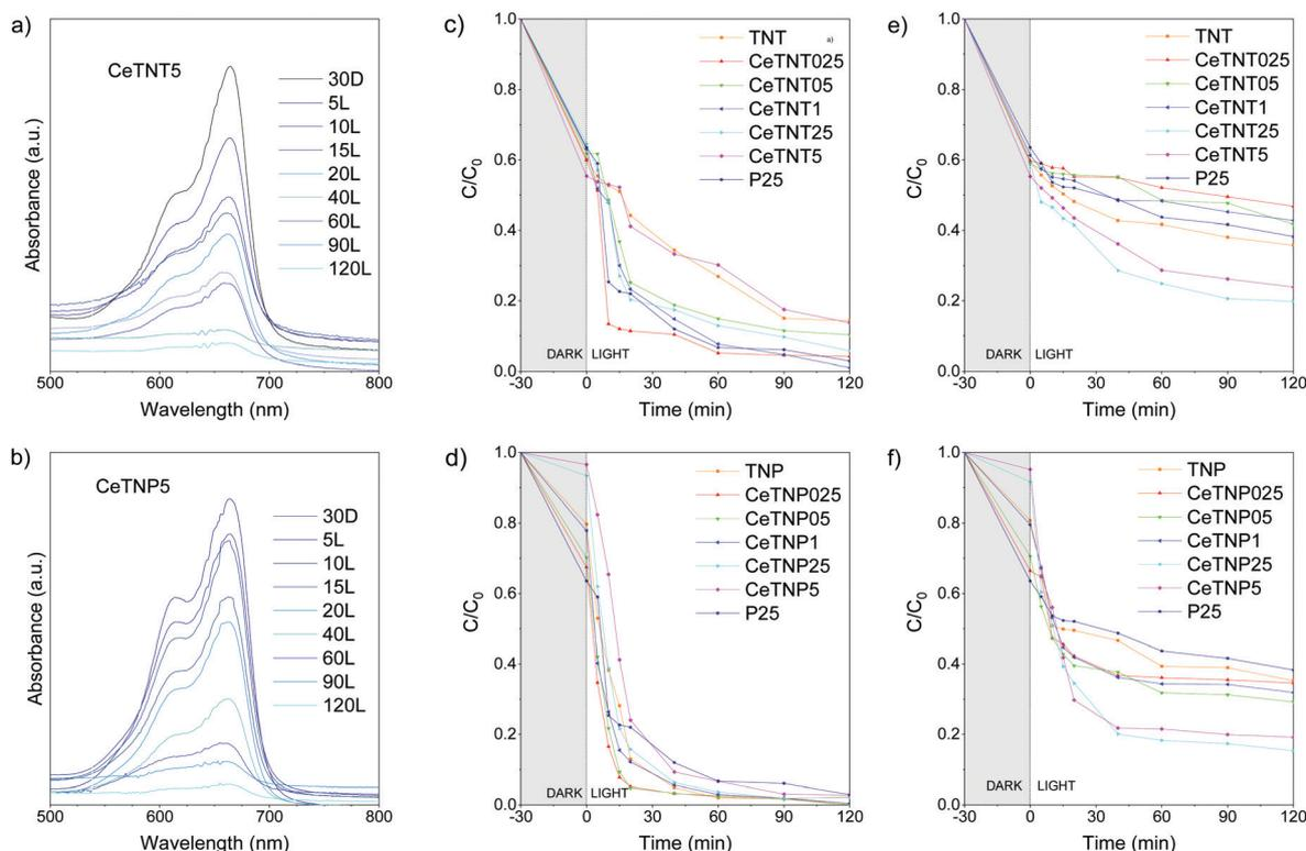
Fig. 4 (a and b) UV-Visible spectra recorded at different times, from 30 min under dark conditions (30D) to 120 min under UV light irradiation (120L), for the two 5.0 wt% CeO<sub>2</sub>-TiO<sub>2</sub> nanostructures: (a) CeTNT5 sample and (b) CeTNP5 sample. (c–f) MB photodegradation test in aqueous solution: CeTNTx (c) under UV light irradiation and (e) under simulated solar light; and CeTNP<sub>x</sub> (d) under UV light irradiation and (f) under simulated solar light.
