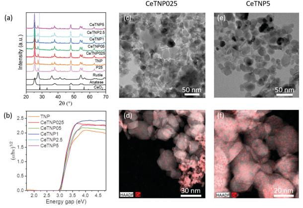
Fig. 2 Undoped and Ce-doped TNP series. (a) XRD patterns, including benchmarking anatase, rutile and P25. (b)  $(\alpha h \nu)^{1/2}$  vs. photoenergy (eV) plot. TEM/ HAADF images for samples CeTNP025 (c and d) and CeTNP5 (e and f). (d) and (f) show the EDS maps for Ce overlapping the STEM images.
