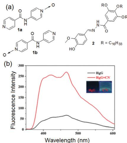
**Fig. 3** (a) Chemical structures of compounds **1a**, **1b** and **2**. (b) Change in the emission of the **2**-Hg<sup>2+</sup> gel (HgG) in the presence of CN<sup>-</sup>. The inset presents the color change of the **2**-Hg<sup>2+</sup> gel (HgG) in the presence of CN<sup>-</sup>. Reproduced from ref. 178 with permission from the Royal Society of Chemistry.
