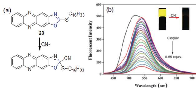
Fig. 19 (a) Chemical reaction involved between **23** and  $\text{CN}^-$  and (b) change in the emission spectra of the DMSO-water gel of **23** in the presence of increasing amounts of  $\text{CN}^-$ . The inset presents the corresponding change in the color of the gel. Adapted with permission from ref. 211.
