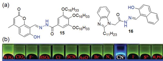
**Fig. 13** (a) Structures of compounds **15** and **16**. (b) Fluorescence response of organogel **16** (WJG) to the presence of various anions. Reproduced from ref. 198 with permission from The Royal Society of Chemistry (RSC) on behalf of the Centre National de la Recherche Scientifique (CNRS) and the RSC.
