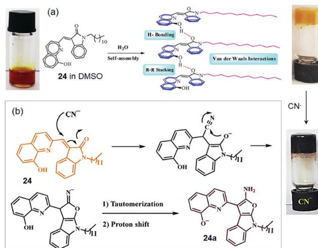
Fig. 20 (a) Suggested self-assembly mechanism for the gel formation of **24** in DMSO/ $\text{H}_2\text{O}$  and (b) a proposed mechanism for the interaction of **24** with  $\text{CN}^-$ . Reproduced with permission from ref. 212.
