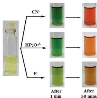
Fig. 18 Photograph showing the colour changes of **22** ( $c = 1.0 \times 10^{-3}$  M) in the presence of equiv. amounts of various anions ( $c = 5.0 \times 10^{-3}$  M) with time in  $\text{CH}_3\text{CN}$  containing 4%  $\text{CHCl}_3$ . Adapted with permission from ref. 210.
