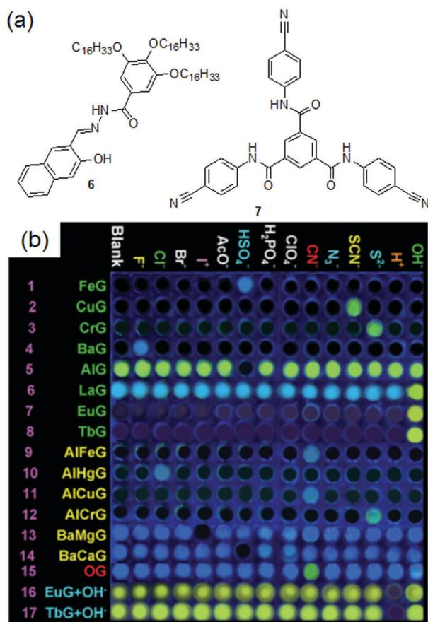
Fig. 7 (a) Structures of compounds 6 and 7. (b) Gel-based sensor array of metallogels of 6 in the presence of various anions. Reproduced from ref. 189 with permission from the Royal Society of Chemistry.
