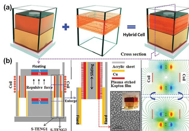
**Fig. 19** (a) Schematic illustration of the hybridized mini-generator for vibration energy harvesting; (b) cross section view of the mini-generator and the simulated magnetic field distribution. Adapted with permission from ref. 100. Copyright 2014 American Chemical Society.
