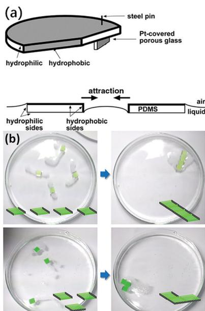
Fig. 25 (a) Design of PDMS plates for self-propulsion and assembly *via* capillary attraction. Adapted with permission from ref. 65. Copyright 2002 Wiley. (b) MSA patterns of line or triangle structures directed by anisotropic modification. Adapted with permission from ref. 32. Copyright 2014 Wiley.
