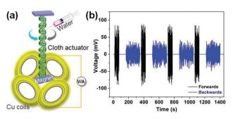
Fig. 13 (a) Schematic illustration of mini-generators based on hygroscopic cloth actuator; (b) induced voltage up to 75 mV produced by the mini-generator. Adapted with permission from ref. 97. Copyright 2017 Wiley.
