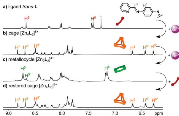
**Fig. 1**  $^1\text{H}$  NMR spectra of (a) ligand *trans*-L (300 MHz,  $\text{CDCl}_3$ ); (b)  $[\text{Zn}_4\text{L}_6](\text{NTf}_2)_8$  cage (300 MHz,  $\text{CD}_3\text{CN}$ ); and (c)  $[\text{Zn}_2\text{L}_2](\text{NTf}_2)_4$  metallo-cycle (300 MHz,  $\text{CD}_3\text{CN}$ ). (d) Interconversion of  $[\text{Zn}_2\text{L}_2](\text{NTf}_2)_4$  into  $[\text{Zn}_4\text{L}_6](\text{NTf}_2)_8$  upon addition of 0.5 equiv. of *trans*-L.
