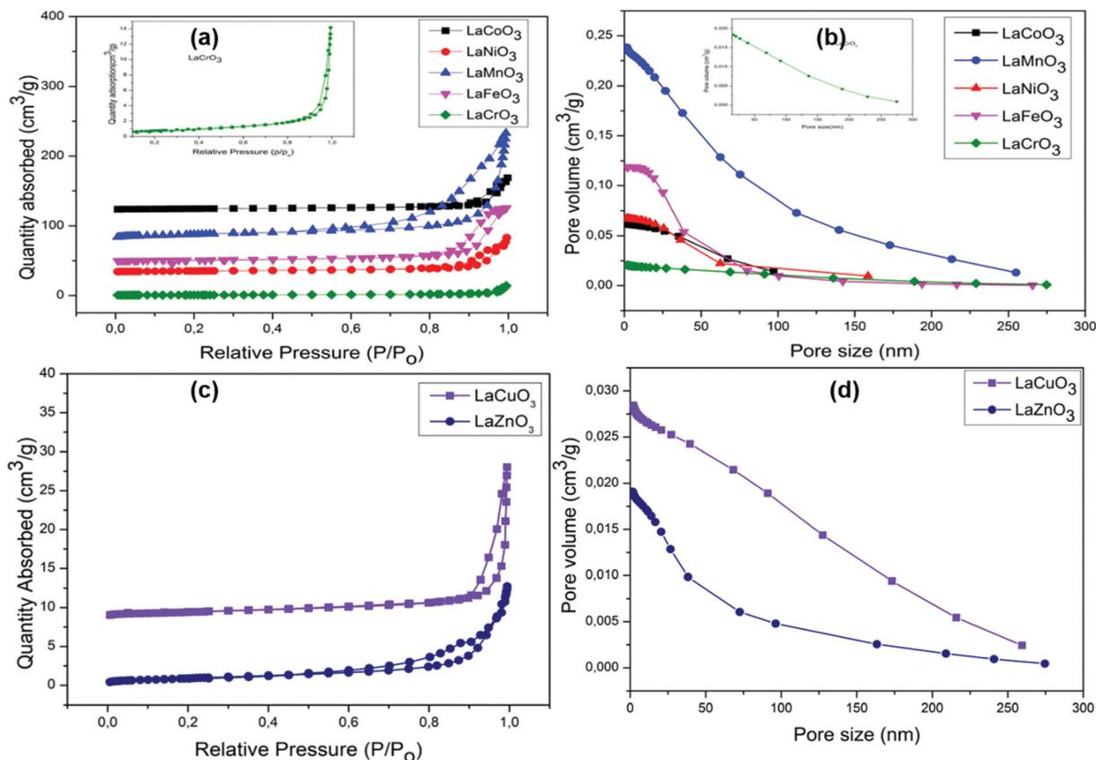
Fig. 5 Plots of (a) nitrogen adsorption–desorption isotherm curves (b) pore volume versus pore size for  $\text{LaMO}_3$  ( $M = \text{Co, Ni, Mn, Fe, Cr}$ ) (c) nitrogen-desorption isotherm curves and (d) pore volume versus pore size for  $\text{LaMO}_3$  ( $M = \text{Cu, Zn}$ ).
