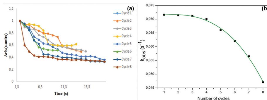
Fig. 9 (a) Absorbance versus time and (b)  $k_{\text{obs}}$  versus number of cycles over LaCrO<sub>3</sub> perovskite.
