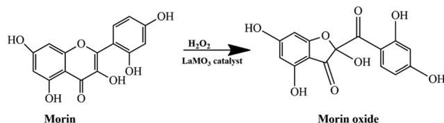
**Scheme 1** Oxidation of morin to morin oxide by  $H_2O_2$  over  $LaMO_3$  ( $M = Co, Cr, Fe, Ni, Mn, Cu, Zn$ ) perovskites.
