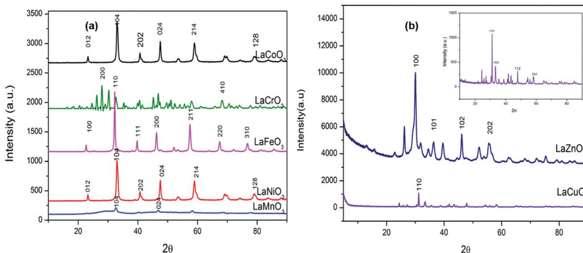
Fig. 1 Wide angle powder X-ray diffraction patterns for (a, b)  $\text{LaMO}_3$  ( $M = \text{Co, Cr, Fe, Ni, Mn, Cu, Zn}$ ) perovskites.
