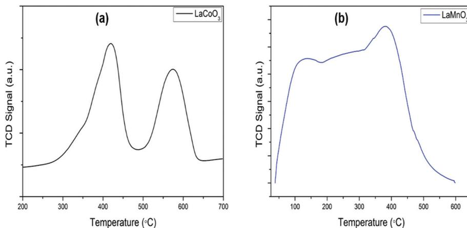
**Fig. 3** TPR profiles for LaCoO<sub>3</sub> and LaMnO<sub>3</sub> perovskites.
