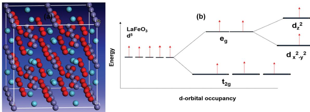
Fig. 7 (a) Optimized structure obtained from material studio and (b) orbital splitting diagram for LaFeO<sub>3</sub> perovskite.
