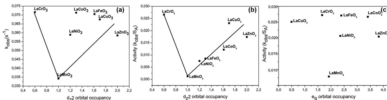
Fig. 8 Plots of (a) reaction rate constant versus  $d_{z^2}$  orbital occupancy, (b) catalytic activity versus  $d_{z^2}$  orbital occupancy with surface area normalised observed rates and (c) catalytic activity versus  $e_g$  orbital occupancy.
