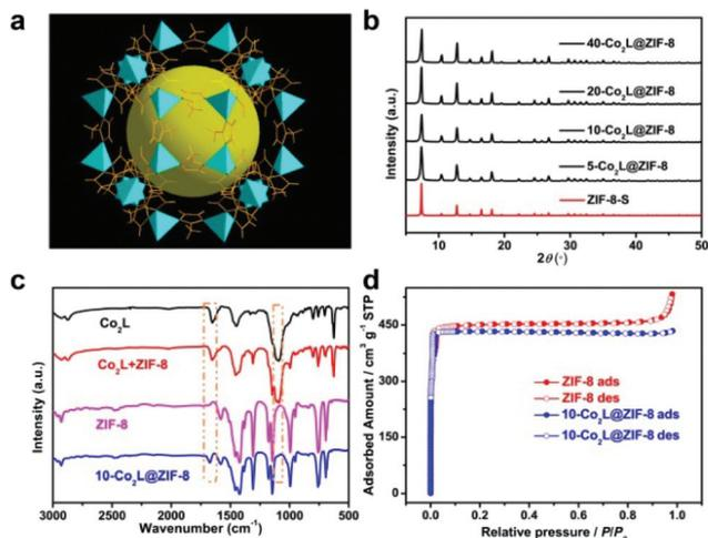
**Fig. 1** (a) Cage structure of  $\text{Co}_2\text{L}@ZIF-8$ . (b) PXRD patterns of  $x\text{-Co}_2\text{L}@ZIF-8$ . (c) FT-IR spectra of  $\text{Co}_2\text{L}$ , ZIF-8, physically mixed  $\text{Co}_2\text{L} + \text{ZIF-8}$ , and host-guest  $\text{Co}_2\text{L}@ZIF-8$ . (d)  $\text{N}_2$  adsorption isotherms of ZIF-8 and  $10\text{-Co}_2\text{L}@ZIF-8$  at 77 K.
