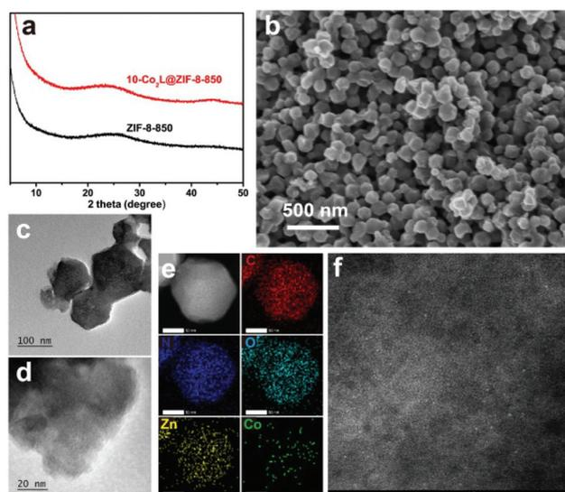
**Fig. 2** (a) PXRD patterns of  $10\text{-Co}_2\text{L@ZIF-8}$  and ZIF-8-850. (b) SEM and (c, d) TEM images of  $10\text{-Co}_2\text{L@ZIF-8-850}$ . (e) HRTEM images and the corresponding elemental mapping of  $10\text{-Co}_2\text{L@ZIF-8-850}$ . (f) HAADF-STEM images of  $10\text{-Co}_2\text{L@ZIF-8-850}$ .
