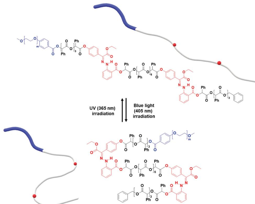
**Fig. 6** Photo-induced isomerization of two photoswitches in the hydrophobic chain of PEG1000-*b*-[OPLA<sub>4</sub>-H1-OPLA<sub>8</sub>-H1-OPLA<sub>4</sub>].
