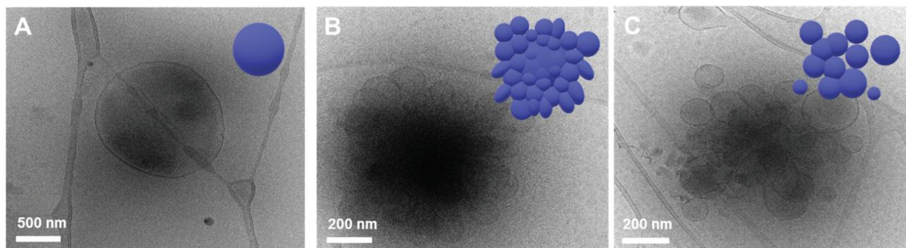
Fig. 4 Cryo-TEM images and 3D graphic representations of self-assembled structures of PEG550-*b*-[OPLA<sub>8</sub>-H1-OPLA<sub>9</sub>] under different light sources. The morphologies were observed (A) before and (B) after blue-light irradiation, followed by (C) UV light irradiation.
