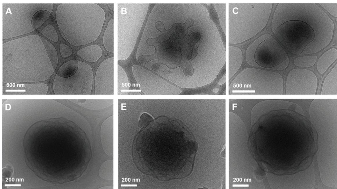
**Fig. 5** Cryo-TEM images of self-assembled structures of (A–C) PEG1000-*b*-[OPLA<sub>8</sub>-H1-OPLA<sub>9</sub>] and (D–F) PEG1000-*b*-[H1-OPLA<sub>17</sub>] under different light sources. The morphologies were observed (A and D) before and (B and E) after blue light irradiation, followed by (C and F) UV light irradiation.
