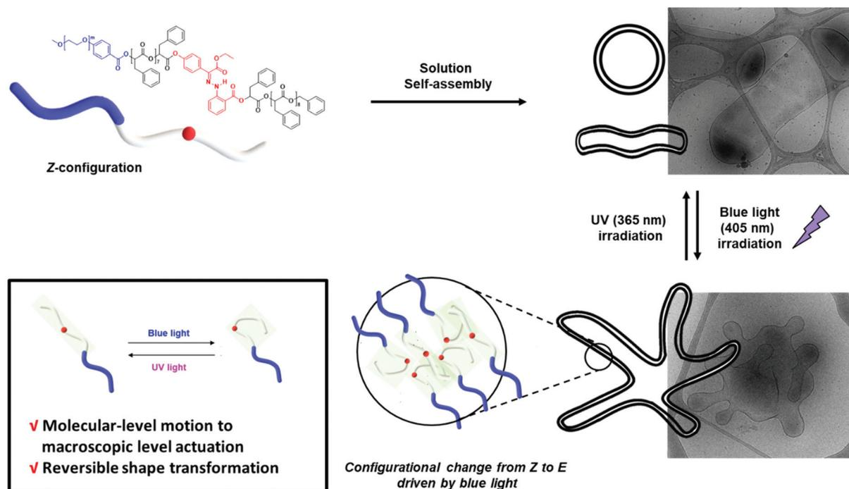
**Fig. 1** Schematic representation of the reversible shape transformation of self-assembled structures of PEG-*b*-[OPLA] containing hydrazone-based photoswitches via configurational switching of the system.
