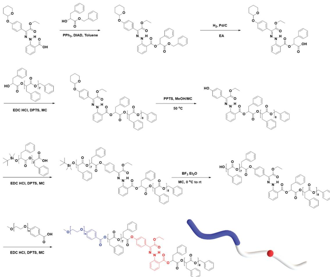
Scheme 2 Synthesis of BCP having hydrazone-based photo-switches (PEG-*b*-[OPLA<sub>8</sub>-H1-OPLA<sub>9</sub>]).
