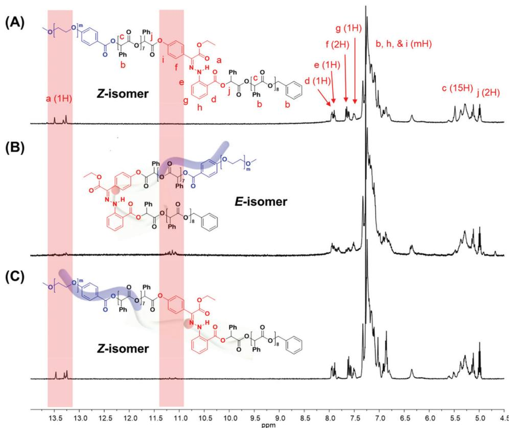
**Fig. 3** <sup>1</sup>H NMR spectra of amphiphilic block copolymer containing hydrazone-based photoswitches (A) before and (B) after irradiation with blue light (405 nm), followed by (C) photoirradiation with UV light (365 nm).
