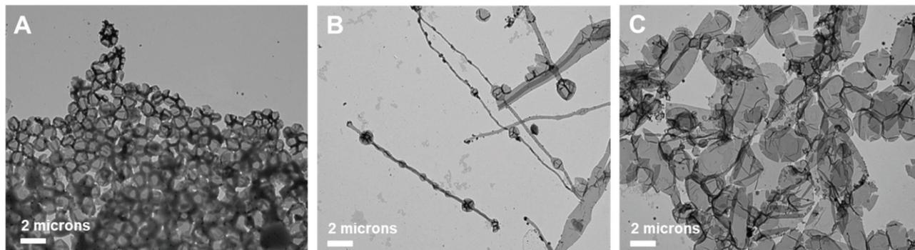
**Fig. 7** TEM images of self-assembled structures of PEG1000-*b*-[OPLA<sub>4</sub>-H1-OPLA<sub>8</sub>-H1-OPLA<sub>4</sub>] under different light sources. The morphologies were observed (A) before and (B) after blue-light irradiation, followed by (C) UV light irradiation. The PEG1000-*b*-[OPLA<sub>4</sub>-H1-OPLA<sub>8</sub>-H1-OPLA<sub>4</sub>] samples were treated with phosphotungstic acid solution for negative staining.
