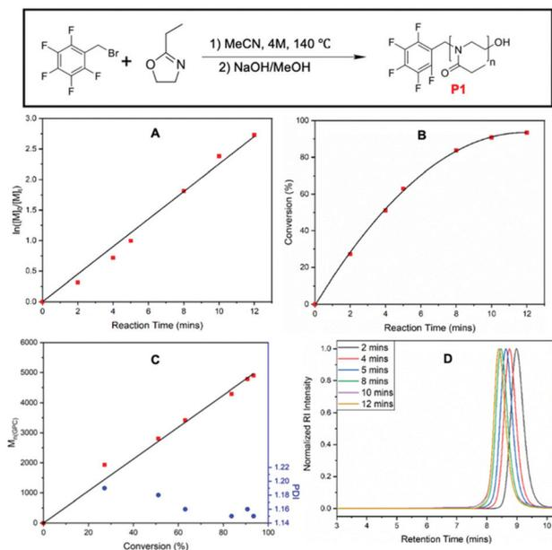
**Fig. 1** Kinetics investigation of PFBB initiated CROP of EtOx. (A)  $\ln([M]_0/[M]_t)$  versus reaction time plot, (B) Monomer conversion versus reaction time plot, (C)  $M_{n,SEC}$  versus monomer conversion and (D) SEC monitored hydrodynamic volume change through the kinetics investigation.
