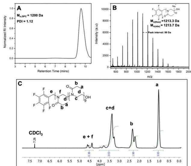
**Fig. 2** (A) SEC measurement in THF as an eluent, (B) MALDI-ToF MS, and (C)  $^1\text{H}$  NMR analysis of PFB-PETox<sub>10</sub>. The SEC trace and the distribution shown in MALDI-ToF indicates a DP10 polymer. In the  $^1\text{H}$  NMR, corresponding peaks were labelled, and part of the backbone hydrogens (f) shifted to lower field at around 4.5 ppm from c+d at 3.45 ppm due to initiating group effect.
