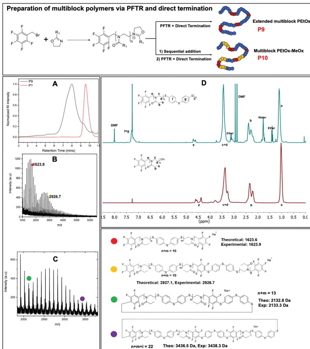
Fig. 4 Preparation of multiblock PETox and characterization of extended multiblock polymer P9 with SEC (A), MALDI-ToF MS (B), zoom in to the high molar mass region in the MALDI-ToF MS (C), and <sup>1</sup>H NMR (D) showing the growth of multiblock polymer and possible cyclic structure formation (green and purple).
