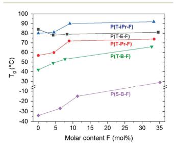
Fig. 5 Influence of the molar content of ferulate units F on the  $T_{\alpha}$  of the terpolyester series.
