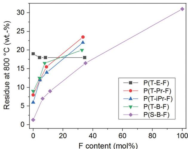
Fig. 7 Influence of the molar content of F units on the residue after TGA at 800 °C.
