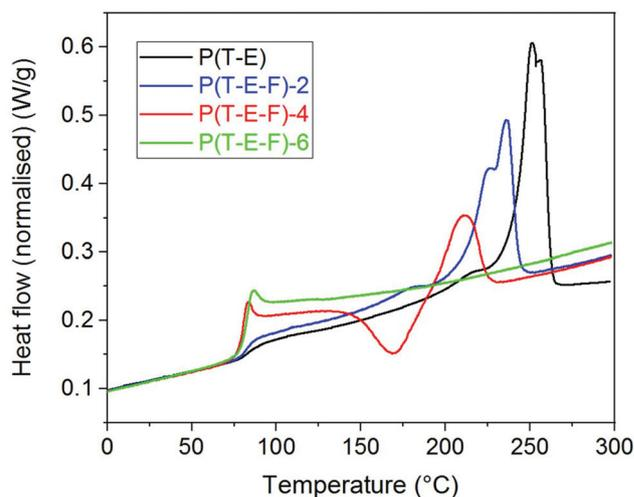
Fig. 4 DSC curves (2<sup>nd</sup> heating) of the terpolyesters P(T-E-F) with different molar content of F.
