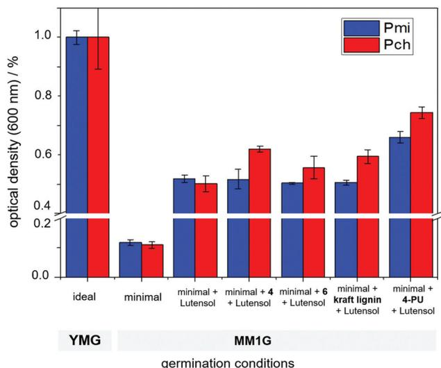
**Fig. 5** Germination of fungal spores of Pmi and Pch quantified from the optical density (measured at 600 nm after 72 h) in YMG (yeast–malt extract plus glucose) or MM1G (minimal growth medium) medium with added particles of **4**, **6**, **4-PU**, or Kraft lignin, stabilized by lutensol. An increase of the optical density indicates stronger mycelium growth and degradation of the added materials.
