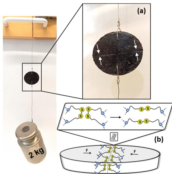
**Fig. 6** Healing of the PA CANs. (a) A disk of Cys60 can withstand a 2 kg load after being cut in half and reconnected by pressing and heating the cut surfaces, the white arrows in the enlarged image point the cut; (b) proposed healing mechanism of the sample through heat-activated disulfide exchange at the interface of the two pieces,  $F$  denotes the force that keeps the two sides in contact with each other.
