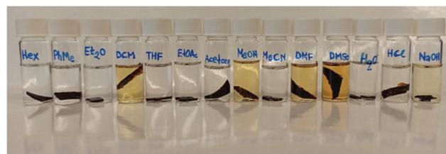
**Fig. 7** Chemical resistance of the PA CANs; Cys40 after being immersed in each solvent for 24 h. From left to right: hexane, toluene, diethyl ether, dichloromethane, tetrahydrofuran, ethyl acetate, acetone, methanol, acetonitrile, dimethylformamide, dimethyl sulfoxide, water, hydrochloric acid (aq. 1 M) and sodium hydroxide (aq. 1 M).
