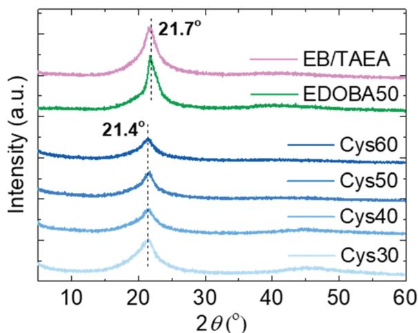
Fig. 3 XRD patterns of the PA CANs and the control networks.
