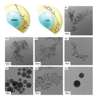
Fig. 1 Scheme for the preparation of polyurea nanocapsules with either DMSO or water as core and transmission electron micrographs of polyurea (P1-5) and polyurethane (P6-7) nanocapsules and nanoparticles.
