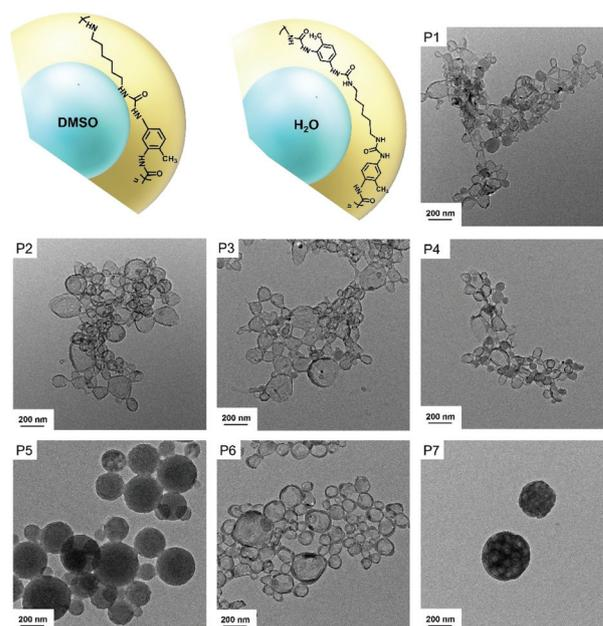
**Fig. 1** Scheme for the preparation of polyurea nanocapsules with either DMSO or water as core and transmission electron micrographs of polyurea (P1–5) and polyurethane (P6–7) nanocapsules and nanoparticles.
