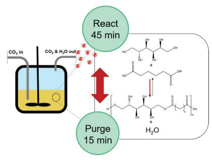
Fig. 2 Schematic representation of the condensation polymerisation of adipic acid with D-Sorbitol in  $scCO_2$  in a reactor vessel. The reactor is filled with  $CO_2$  through an inlet while  $CO_2$  and  $CO_2$  and  $CO_2$  and  $CO_2$  and  $CO_2$  and  $CO_2$  and  $CO_2$  are through the outlet on the right when the reactor is purged.
