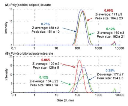
Fig. 6 DLS measurement of (A) poly(sorbitol adipate) laurate and (B) poly(sorbitol adipate) stearate at increasing concentrations 0.06 (-), 0.12 (-) and 0.25 (-) wt%, plotting size distribution (d, nm) by intensity. Note the increase in size for the stearate derivative, whereas the laurate polyester remains relatively constant. Peaks at higher hydrodynamic volumes (<2%) are thought to be caused by dust particles interfering with the reading.
