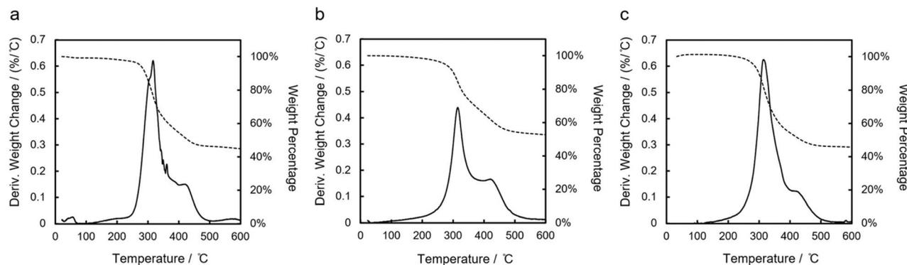
Fig. 5 TGA curves of (a) *lin*-poly(1,4Si<sub>6</sub>), (b) *cyc*-poly(1,3Si<sub>6</sub>) and (c) *lin*-poly(1,3Si<sub>6</sub>). Solid lines: derivative weight change; dotted lines: percentage weight change.
