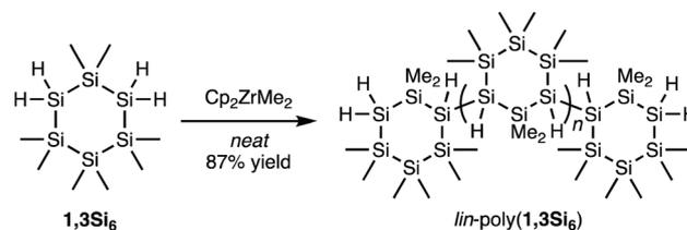
Scheme 1 Synthesis of *lin*-poly(**1,3Si**<sub>6</sub>), a linear polymer of **1,3Si**<sub>6</sub>.
