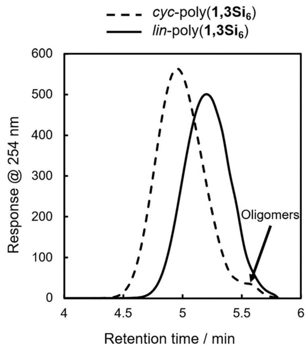
Fig. 2 GPC of *cyc*-poly(**1,3Si**<sub>6</sub>) (dotted line) and *lin*-poly(**1,3Si**<sub>6</sub>) (solid line). Determined relative to polystyrene standards at 254 nm (THF, [*lin*-poly(**1,3Si**<sub>6</sub>)] = 1 mg mL<sup>-1</sup>, 40 °C, 0.35 mL min<sup>-1</sup>, 10 μL injection).
