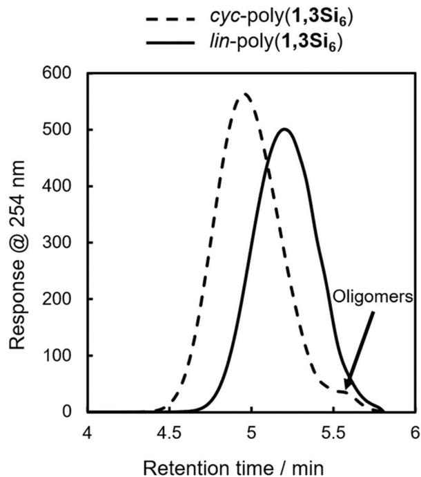
Fig. 2 GPC of *cyc*-poly(**1,3Si<sub>6</sub>**) (dotted line) and *lin*-poly(**1,3Si<sub>6</sub>**) (solid line). Determined relative to polystyrene standards at 254 nm (THF, [**1,3Si<sub>6</sub>**] = 1 mg mL<sup>-1</sup>, 40 °C, 0.35 mL min<sup>-1</sup>, 10 μL injection).
