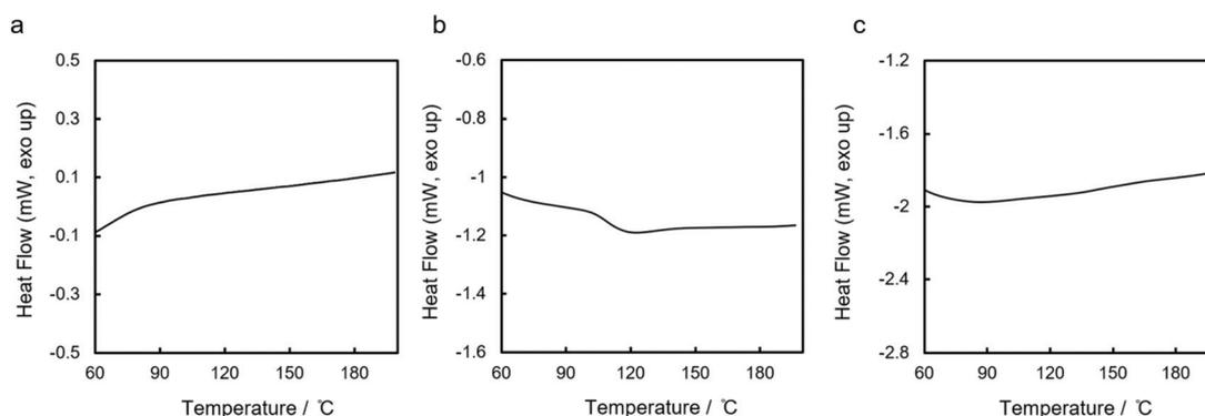
Fig. 4 DSC curves of (a) *lin*-poly( $1,4\text{Si}_6$ ), (b) *cyc*-poly( $1,3\text{Si}_6$ ), and (c) *lin*-poly( $1,3\text{Si}_6$ ). The second cycle is shown. Heating rate: 3 °C  $\text{min}^{-1}$  for *lin*-poly( $1,4\text{Si}_6$ ), 20 °C  $\text{min}^{-1}$  for *cyc*-poly( $1,3\text{Si}_6$ ) and *lin*-poly( $1,3\text{Si}_6$ ).
