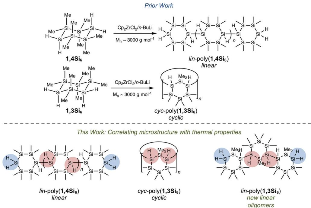
**Fig. 1** (a) Prior work:  $\text{Cp}_2\text{ZrCl}_2/n\text{-BuLi}$ -mediated dehydrocoupling polymerization of directional building blocks  $1,4\text{Si}_6$  and  $1,3\text{Si}_6$ . (b) This work: Synthesis of new linear  $\text{lin-poly}(1,3\text{Si}_6)$  and analysis of relationships between microstructure and thermal decomposition.
