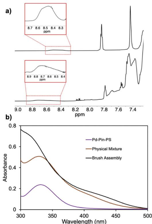
**Fig. 4** (a) <sup>1</sup>H NMR spectroscopic overlay of (top) physical mixture of *co*-PIC and Pd-Pin-PS, and (bottom) assembled *co*-PIC-brush-Pd-Pin-PS after AgBF<sub>4</sub> addition. (b) UV-Vis traces of (purple) Pd-Pin-PS, (brown) physical mixture of *co*-PIC and Pd-Pin-PS, and (black) assembled *co*-PIC-brush-Pd-Pin-PS. (DCE, 25 °C).
