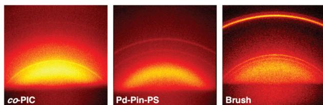
Fig. 7 Two-dimensional diffraction patterns of (left to right) *co*-PIC, Pd-Pin-PS, and brush assembly. The bright peak at wide-angle area in the brush assembly suggests the formation of long-range ordered structures.
