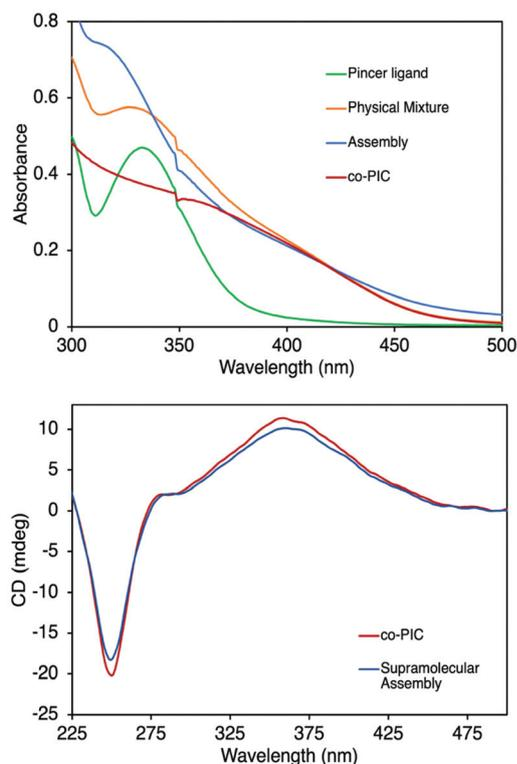
**Fig. 3** Spectroscopic analysis of *co*-PIC assembly with Pd-Pin. (top) UV-Vis traces of (green) Pd-Pin, (red) *co*-PIC, (orange) physical mixture, and (blue) metal coordination after AgBF<sub>4</sub> addition, recorded in DCE at 25 °C with [co-PIC] = 7.5 μM. (bottom) CD traces of (red) *co*-PIC and (blue) metal coordination after AgBF<sub>4</sub> addition, recorded in DCE at 25 °C with [co-PIC] = 7.5 μM.
