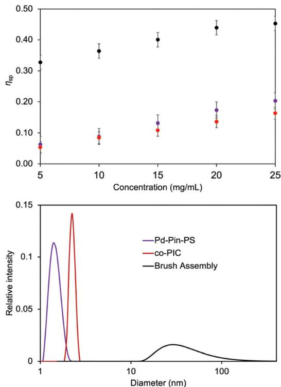
Fig. 6 Characterizing the brush copolymer assembly by measuring (top) specific viscosity ( $\eta_{sp}$ ) in  $\text{CHCl}_3$  and (bottom) hydrodynamic radii ( $R_h$ ) in DMSO; (red) *co-PIC*, (purple) **Pd-Pin-PS**, and (black) supramolecular brush assembly.
