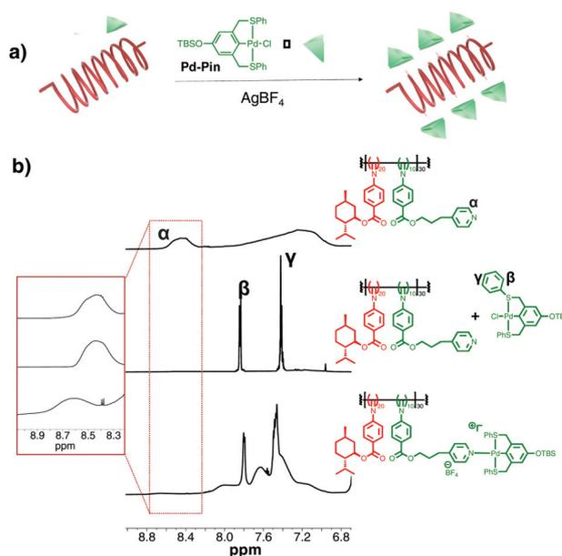
**Fig. 2** (a) Schematic representation of the side-chain supramolecular assembly of **co-PIC** and **Pd-Pin** complex. (b) Partial  $^1\text{H}$  NMR (600 MHz) spectroscopic overlay of (top to bottom) **co-PIC**, physical mixture of **co-PIC** and **Pd-Pin**, and metal coordination assembly after  $\text{AgBF}_4$  addition.
