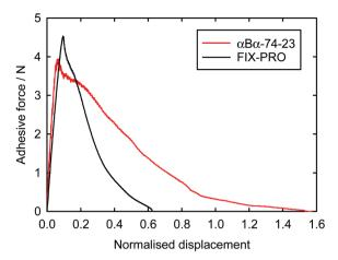
Fig. 6 Representative probe adhesion results for single specimens of  $\alpha B\alpha$ -74-23 and FIX-PRO® to full detachment. W=69.3 kJ m $^{-3}$  for  $\alpha B\alpha$ -74-23, and 39.5 kJ m $^{-3}$  for FIX-PRO® were determined from the areas under the curves.
