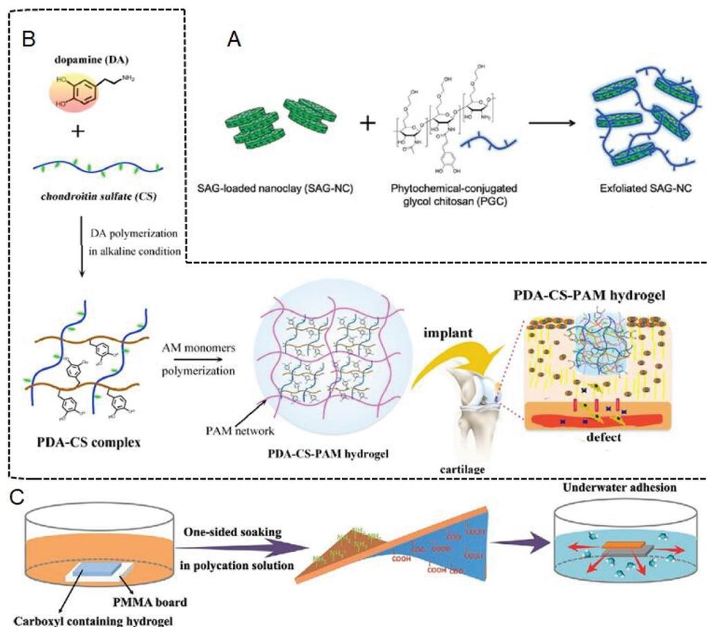
Fig. 7 (A) Schematic diagram of NoBS. Figure reproduced with permission from Wiley.<sup>121</sup> (B) Schematic diagram of PDA–CS–PAM. Figure reproduced with permission from American Chemical Society.<sup>164</sup> (C) Schematic diagram of the Janus hydrogel formed by immersing one side of a carboxyl-containing self-adhesive hydrogel in a polycation solution and complexing with the gradient polyelectrolyte. Figure reproduced with permission from Wiley.<sup>169</sup>
