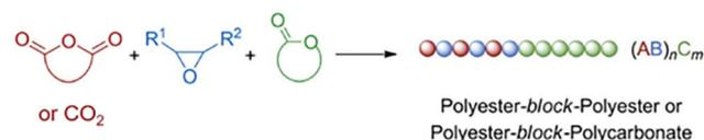
**Fig. 14** One-shot switchable copolymerization of epoxide, anhydride (CO<sub>2</sub>) and lactone using a dizinc catalyst, obtaining polyester (polycarbonate)-*b*-polyester block copolymers by sequential ROCOP of epoxides/anhydrides (CO<sub>2</sub>) and ROP of lactones.
