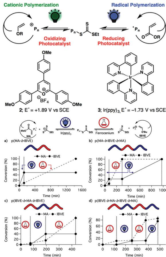
**Fig. 8** The switchable controlled/living radical and cationic copolymerizations with orthogonal stimuli. Reproduced from ref. 33 and 34 with permission from the American Chemical Society, copyright 2017 and 2018.
