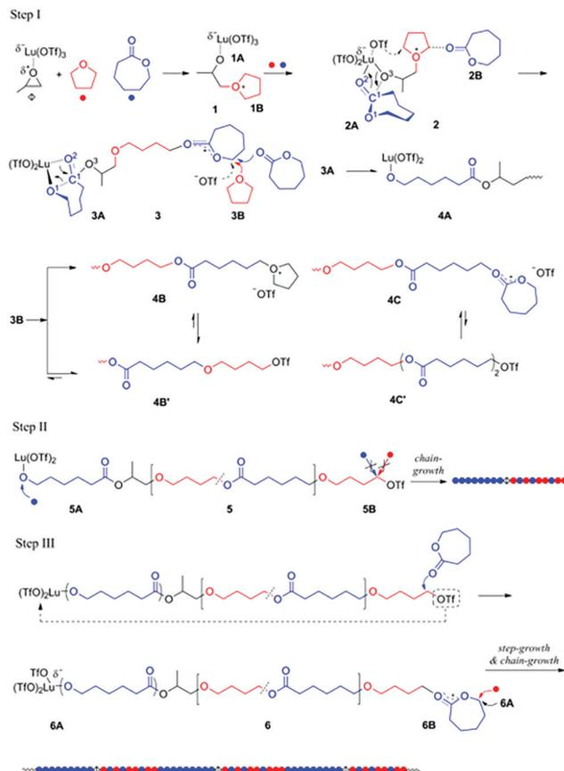
**Fig. 6** Hybridization of cationic and anionic copolymerizations catalyzed by Lu(OTf)<sub>3</sub>/PO. Reproduced from ref. 26 with permission from the American Chemical Society, copyright 2014.
