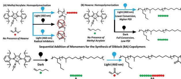
**Fig. 7** The switchable copolymerization converting from coordination–insertion polymerization of hexene to radical polymerization of methacrylate in one shot under visible light irradiation. Reproduced from ref. 31 with permission from the American Chemical Society, copyright 2018.
