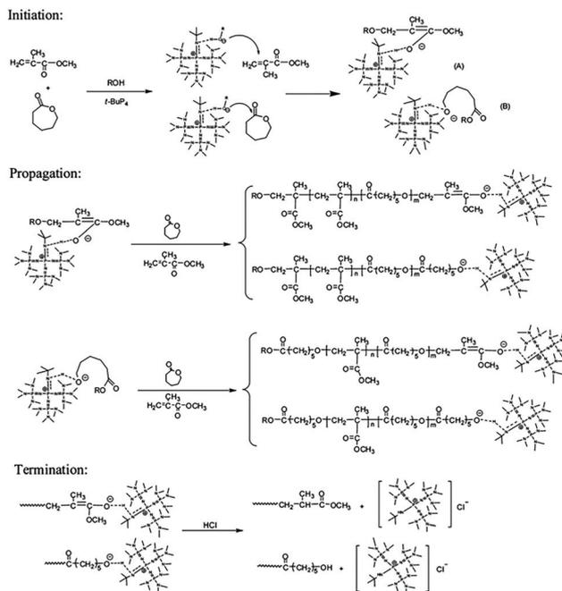
Fig. 1 Hybridization of anionic addition polymerization of MMA and anionic ring-opening polymerization of  $\epsilon$ -caprolactone. Reproduced from ref. 16 with permission from the American Chemical Society, copyright 2012.
