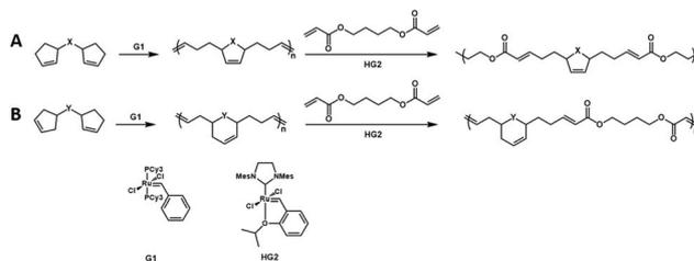
Fig. 17 Cascade metathesis polymerization containing ring-opening, ring-closing, and cross metathesis. (A) Cyclopentene in the main chain. (B) Cyclohexene in the main chain.
