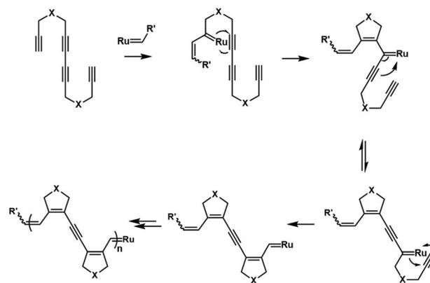
Fig. 18 Cascade olefin metathesis/metallo-tropic 1,3-shift (M&M) polymerization.
