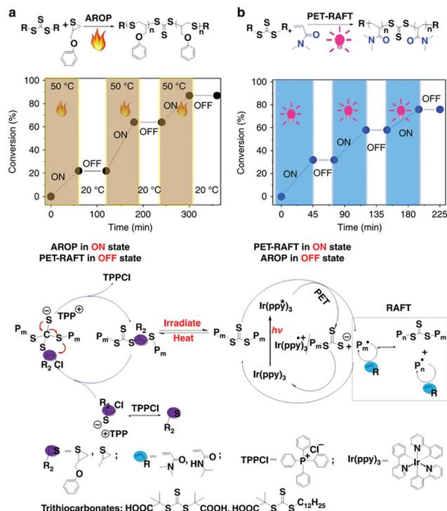
**Fig. 10** Dually switchable and controlled interconvertible copolymerizations of AROP and PET-RAFT switched ON/OFF and interconverted in response to stimuli. Reproduced from ref. 40 with permission from the Nature Publishing Group, copyright 2018.
