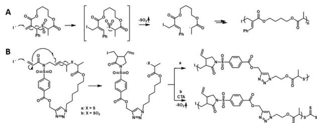
**Fig. 15** (A) Radical-driven ring-opening cascade polymerization enabled by the allylic sulfone trigger. (B) Radical-driven ring-closing/ring-opening cascade polymerization of macrocyclic monomers consisting of 1,6-diene-fused allylic sulfide and sulfone.
