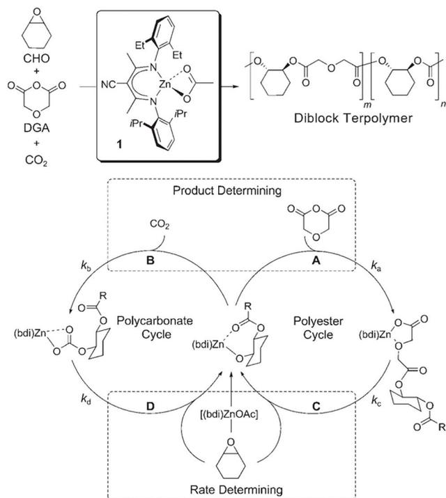
**Fig. 13** One-shot switchable copolymerization of an epoxide, anhydride and CO<sub>2</sub> mixture, obtaining polyester-*b*-polycarbonate block copolymers by sequential ROCOP of epoxides/anhydrides and ROCOP of epoxides/CO<sub>2</sub>. Reproduced from ref. 50 with permission from John Wiley and Sons, copyright 2008.
