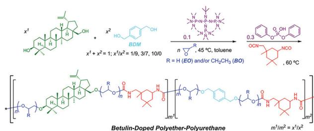
**Fig. 12** One-pot switchable ring-opening polymerization of ethylene oxide and step-growth polymerization of hydroxy and isocyanate. Reproduced from ref. 46 with permission from the American Chemical Society, copyright 2018.
