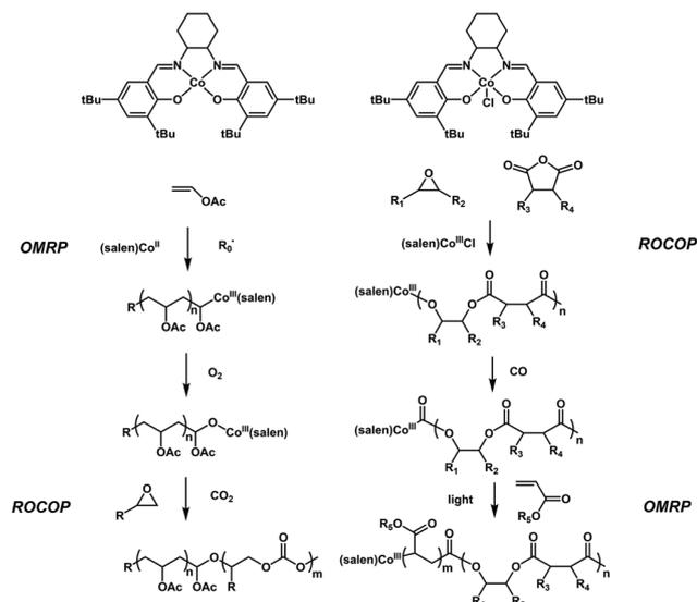
**Fig. 11** (A)  $O_2$ -triggered copolymerization switched from cobalt-mediated OMRP to ROCOP for the synthesis of  $CO_2$ -based diblock copolymers. (B)  $CO$ -triggered copolymerization switched from cobalt-mediated ROCOP to OMRP for the one-pot synthesis of polyester-*b*-polyacrylate.
