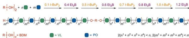
**Fig. 9** Illustration of one-pot synthesis of a multiblock copolymer from a mixture of VL and PO after several successive switches in selectivity. Reproduced from ref. 37 with permission from John Wiley and Sons, copyright 2019.
