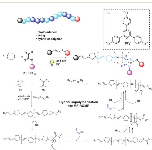
**Fig. 3** Visible-light-induced hybridization of radical addition polymerization of MMA and ROMP of ring-strained cyclic olefins. Reproduced from ref. 22 with permission from the American Chemical Society, copyright 2019.
