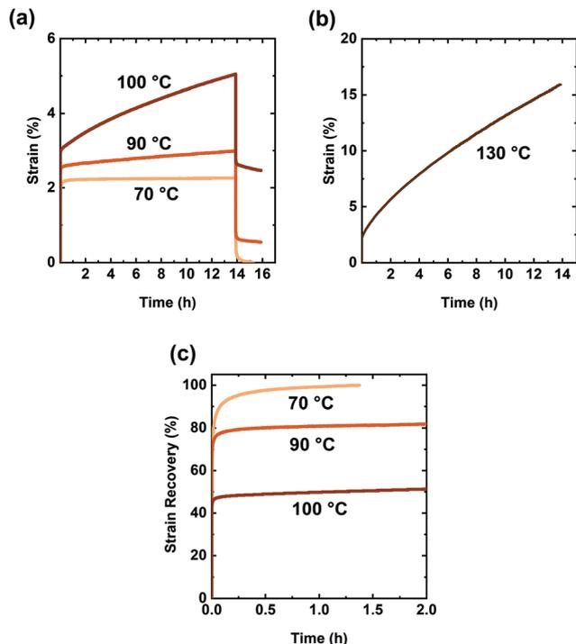
**Fig. 6** (a) Creep and creep recovery curves of the XLPHMA-5 network at different temperatures under a constant stress of 3 kPa. (b) Creep curve of the XLPHMA-5 network at the processing temperature (130 °C) under a constant stress of 3 kPa. (c) Strain recovery as a function of time for the XLPHMA-5 network at different temperatures after 13.9 h of creep testing under a constant stress of 3 kPa.
