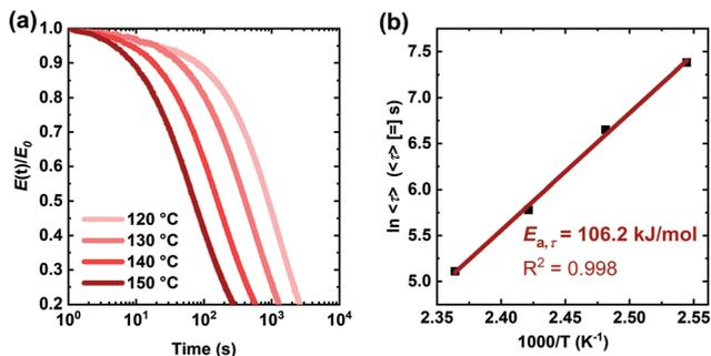
**Fig. 8** (a) Normalized stress relaxation curves of the XLPHMA-5 network at different temperatures under a strain of 5%. (b) Arrhenius apparent activation energy of stress relaxation associated with average relaxation time for the XLPHMA-5 network.
