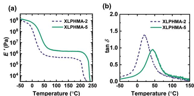
Fig. 2 (a) Tensile storage modulus ( $E'$ ) and (b) damping ratio ( $\tan \delta = E''/E'$ ) of 1<sup>st</sup> mold XLPHMA-2 and XLPHMA-5 networks.
