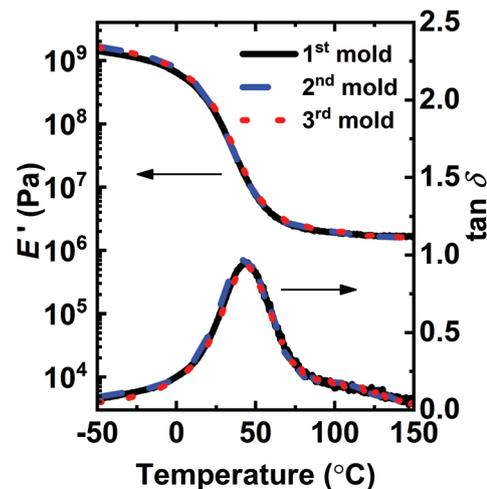
Fig. 3 Tensile storage modulus ( $E'$ ) and damping ratio ( $\tan \delta = E''/E'$ ) of 1<sup>st</sup> mold, 2<sup>nd</sup> mold, and 3<sup>rd</sup> mold XLPHMA-5 network samples.
