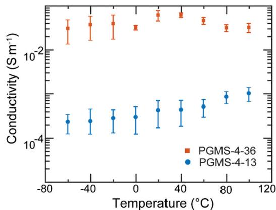
**Fig. 5** Electronic conductivity of PGMS as a function of temperature for a 400 nm channel length. The conductivity of the thin films did not change significantly despite an increase in temperature of >100 K. An increase in radical content increased the conductivity of the thin films from PGMS-4-13 to PGMS-4-36. Each data point represents the average of 4 different PGMS thin film measurements and the error bars represent the standard deviation from the average.
