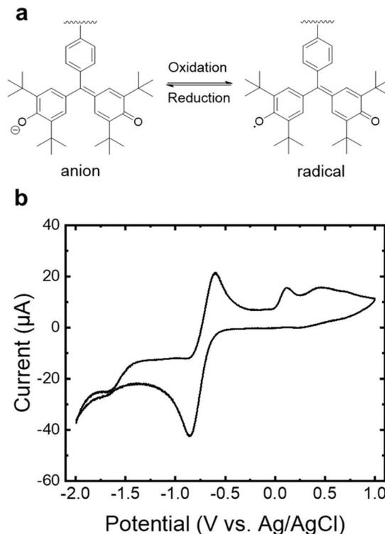
**Fig. 4** (a) The reversible redox reaction of PGMS. (b) Cyclic voltammogram of PGMS-39 (radical content 29%) on a gold working electrode using platinum as the counter electrode, recorded at a scan rate of  $0.1 \text{ V s}^{-1}$  in  $0.1 \text{ M}$  tetrabutylammonium hexafluorophosphate (TBAPF<sub>6</sub>) in *N,N*-dimethylformamide (DMF). The voltammogram shown was obtained after 5 conditioning cycles.
