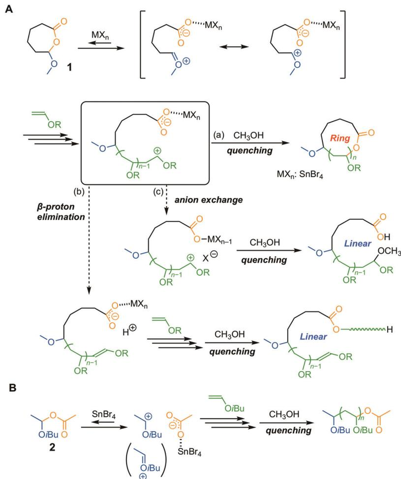
**Fig. 1** (A)  $\text{SnBr}_4$ -catalyzed ring-expansion cationic polymerization of vinyl ether with a cyclic HAE-based initiator (**1**); ideal propagation and termination (a) and unfavorable side reactions (b and c). (B)  $\text{SnBr}_4$ -catalyzed living cationic polymerization of IBVE with an acyclic HAE-based initiator **2** affording an HAE terminal structure.
