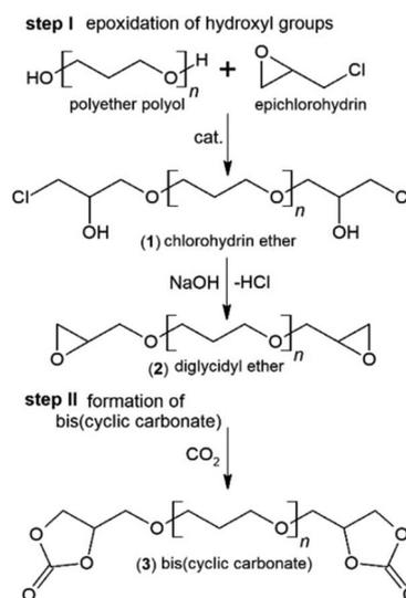
**Fig. 1** Scheme of the reaction between polyether polyol and epichlorohydrin (I step) and cycloaddition of CO<sub>2</sub> into diglycidyl ether (II step).
