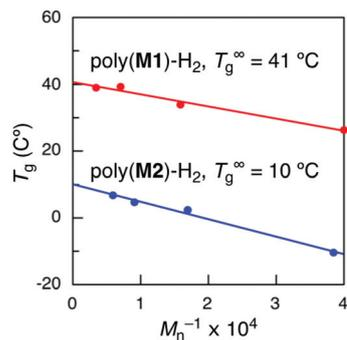
Fig. 6  $T_g$  values of hydrogenated poly(M1) (poly(M1)-H<sub>2</sub>) and poly(M2) (poly(M2)-H<sub>2</sub>) with various molecular weights and  $T_g^\infty$  values estimated using the Flory–Fox equation.
