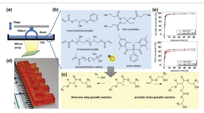
Fig. 1 (a) Schematic representation of DLP process. (b) Monomers and transesterification catalyst used for the preparation of covalent adaptable thiol—acrylate photopolymers. (c) Schematic representation of the photo-curing reaction. (d) Photograph of a 3D printed test structure with a length of 2.6 cm. (e) Curing kinetics as obtained from FTIR data. The lines are a guide for the eye.
