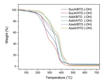
Fig. 5 TGA thermograms of hydroxyl-terminated branched polyesters.
