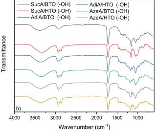
**Fig. 1** FT-IR spectra of branched polyesters bearing: (a) terminal carboxyl, and (b) terminal hydroxyl groups.
