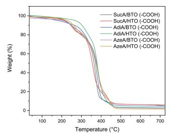
Fig. 4 TGA thermograms of carboxyl-terminated branched polyesters.
