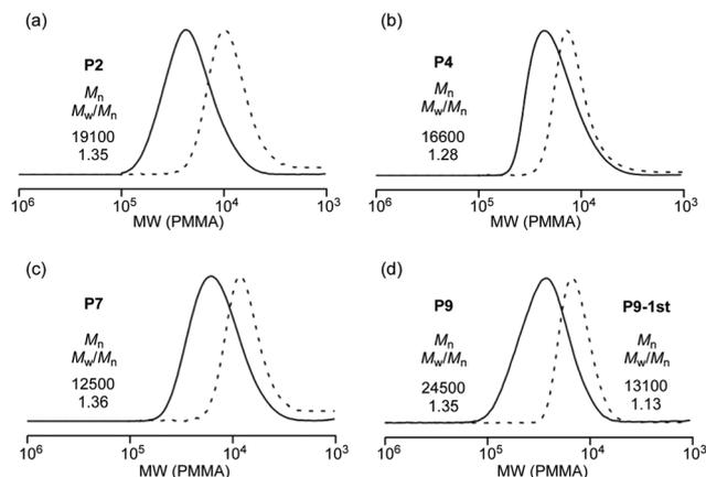
Fig. 2 SEC curves of (a) **P2**, (b) **P4**, (c) **P7**, their intermediates obtained at earlier conversion (dashed lines, PEGA/ODA + OLA conversion = (a) 16%/16%, (b) 20%/21%, and (c) 12%/12%), and (d) **P9** and **P9-1st** (macroinitiator, dashed line).
