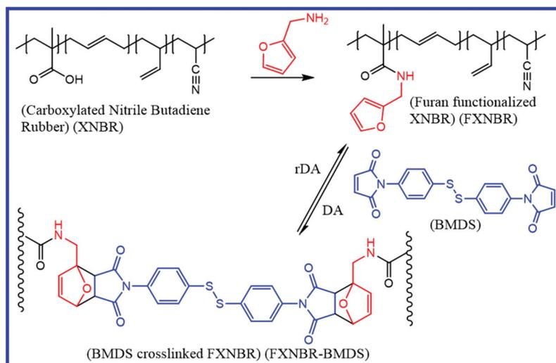
Fig. 22 Schematic representation of the preparation of self-healing XNBR having disulfide moiety and DA bond.<sup>141</sup>
