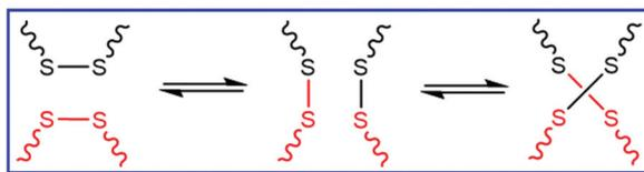
Fig. 6 Schematic representation of the disulfide metathesis reaction.
