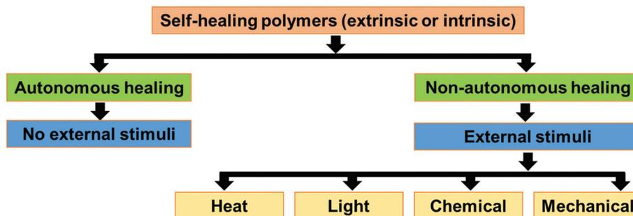
Fig. 2 Classification of self-healing polymers based on the stimuli required for the healing process.
