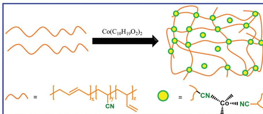
Fig. 21 Schematic representation of the preparation of coordination crosslinked NBR.<sup>136</sup>
