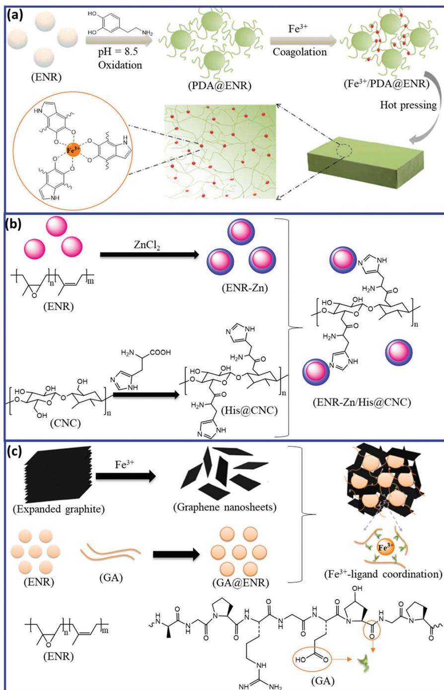
**Fig. 15** Schematic representation of the preparation of self-healing ENR via reversible coordinate bonds; (a) catechol-Fe<sup>3+</sup>, (b) histidine-Zn<sup>2+</sup>, and (c) gelatine-Fe<sup>3+</sup>.<sup>96–98</sup> Reproduced from ref. 96 with permission from American Chemical Society, copyright 2017. Reproduced from ref. 98 with permission from American Chemical Society, copyright 2019.
