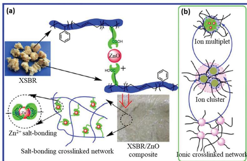
Fig. 9 (a) Schematic representation of network formation by the reaction between carboxyl groups of XNBR and zinc oxide. (b) Schematic for ion multiplet, ion cluster, and ionic crosslinked network.<sup>79</sup> Reproduced from ref. 79 with permission from American Chemical Society, copyright 2016.
