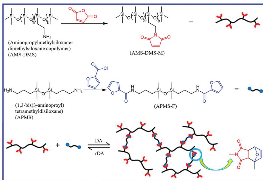
Fig. 23 Schematic representation of the preparation of the self-healing polysiloxane elastomer with DA bonds.<sup>155</sup> Reproduced from ref. 155 with permission from Royal Society of Chemistry, copyright 2016.
