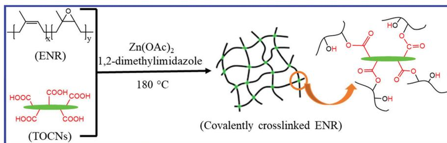
Fig. 18 Schematic representation of the preparation of TOCNs cross-linked ENR *via* the epoxy-acid reaction<sup>112</sup> Reproduced from ref. 112 with permission from Royal Society of Chemistry, copyright 2019.
