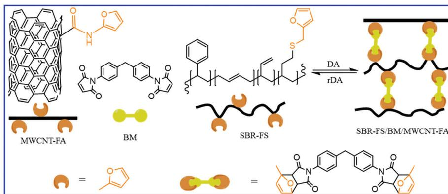
Fig. 11 Schematic representation for the preparation self-healable SBR-FS/BM/MWCNT-FA nanocomposites *via* DA reaction of the furan group of rubber and CNT with bismaleimide.<sup>81</sup>
