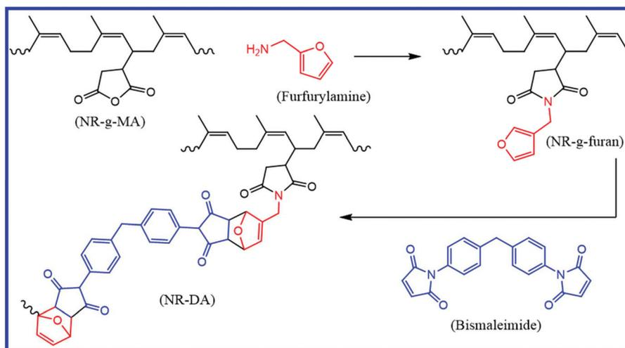
**Fig. 12** Schematic representation of the preparation of furan-functionalized NR and the crosslinking of furan-functionalized NR via the DA reaction using bismaleimide.<sup>85</sup> Reproduced from ref. 85 with permission from Elsevier, copyright 2019.
