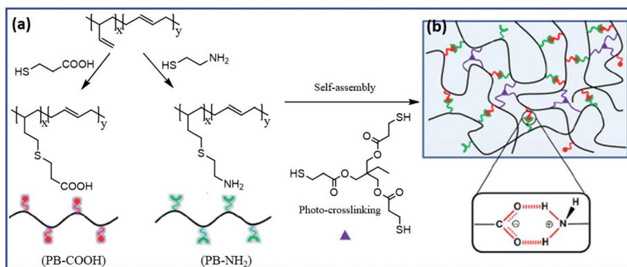
Fig. 8 (a) Schematic representation of the preparation of  $-\text{COOH}$  and  $-\text{NH}_2$  functionalized PB *via* the thiol-ene reaction. (b) The polymer network having both ionic hydrogen bonds and covalent cross-links.<sup>73</sup> Reproduced from ref. 73 with permission from Royal Society of Chemistry, copyright 2015.
