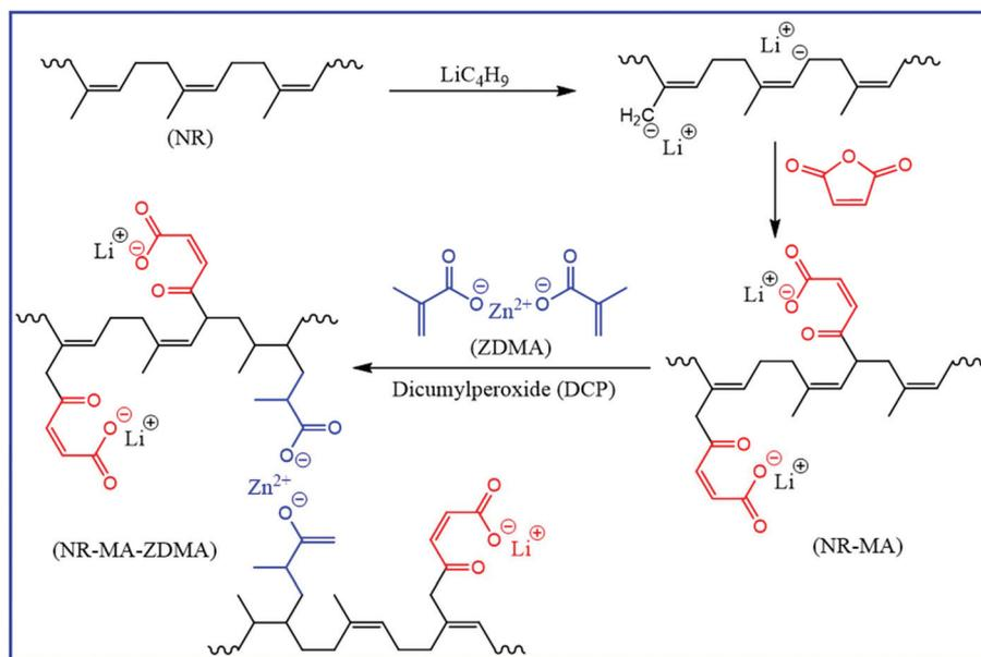
Fig. 14 Schematic representation of the preparation of self-healing NR having a dual ionic network.<sup>92</sup> Reproduced from ref. 92 with permission from American Chemical Society, copyright 2020.
