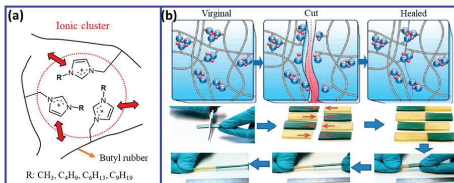
**Fig. 20** (a) Schematic representation of the formation of the ionic cluster in the imidazole-modified BIIR.<sup>127</sup> (b) Dissociation and association ionic groups during the self-healing process.<sup>126</sup> Reproduced from ref. 126 with permission from American Chemical Society, copyright 2015. Reproduced from ref. 127 with permission from American Chemical Society, copyright 2017.
