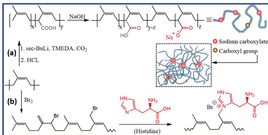
**Fig. 13** (a) Schematic illustration of the preparation of sodium carboxylate-functionalized IR and ionic association in it.<sup>86</sup> (b) Schematic representation of the preparation of self-healing NR ionomer from brominated NR.<sup>89</sup> Reproduced from ref. 86 with permission from Springer Nature, copyright 2019. Reproduced from ref. 89 with permission from Elsevier, copyright 2020.
