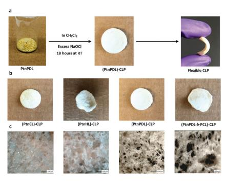
Fig. 3 (a) Image of PtnPDL-CLP flexible polymer. (b) Images of PtnCL, PtnHL, and P(tnPDL-b-CL) CLPs (c) Cross sectional morphology of crosslinked polymers under optical microscopy; magnification ×10.
