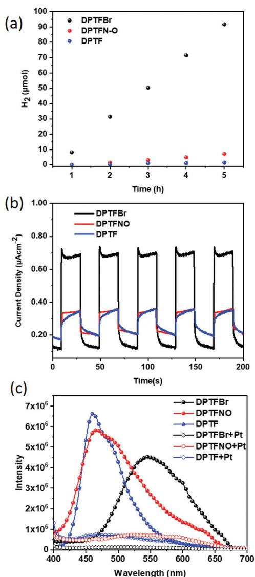
Fig. 5 (a) Photocatalytic hydrogen evolution data from DPTF, DPTFBr, and DPTFNO. (b) The photocurrent responses of the conjugated polymers at an applied voltage of 0 V (with 0.1 M  $\text{Na}_2\text{SO}_4$  as the electrolyte). (c) PL spectra of CPEs with or without 3% Pt cocatalyst.
