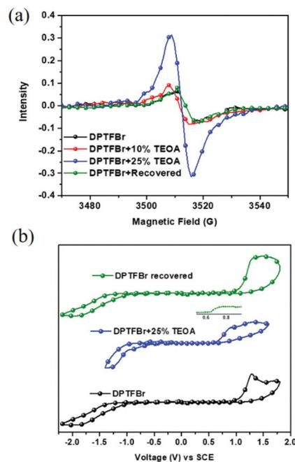
**Fig. 3** (a) ESR spectra of DPTFBr samples with 0 wt%, 10 wt%, and 25 wt% TEOA (illuminated for 30 min) and a recovered sample. (b) CV curves of pure DPTFBr, DPTFBr with 25% TEOA, and recovered DPTFBr samples.
