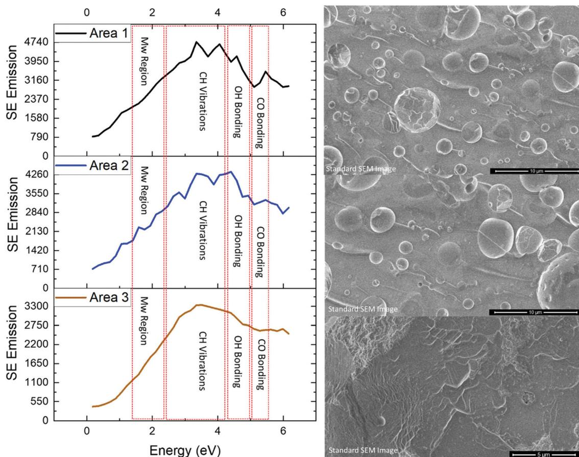
**Fig. 1** Secondary electron spectra with accompanying SEM images for PR382 area 1, 2 and 3 highlighting SE regions identified as associated with functional group emissions. Area 1 & 2 HFW = 30 μm whereas area 3 HFW = 25 μm.
