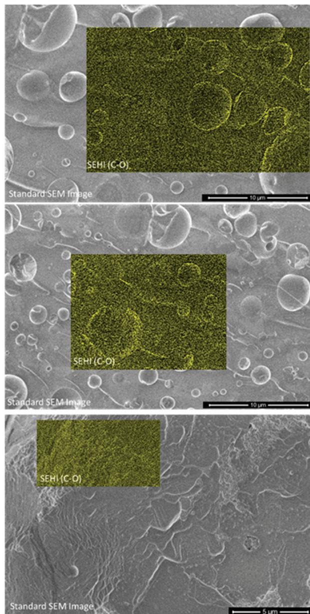
**Fig. 4** SEHI images generated from the component analysis of PR382 mapping CO bonding (indicating ether bridge distributions). With the stronger emission intensity showing greater CO bonding. SEHI images are overlaid with grayscale standard SE images (integral over all energy ranges) of PR382.
