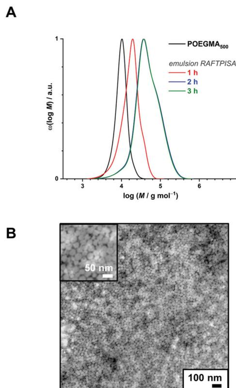
**Fig. 2** (A) Size-exclusion chromatograms of polymers obtained by PBBMA emulsion RAFTPISA in water/ethanol 3 : 1 vol/vol at 70 °C with POEGMA<sub>500</sub> at  $DP_{th} = 100$ , and 20 wt% solids content (entry 4 from Table S2<sup>†</sup>). (B) Transmission electron micrograph of nanoparticles obtained in the conditions mentioned above, after 2 h.
