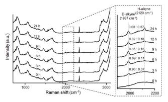
Fig. 4 Average Raman spectra of the lipid region ( $20 \times 20$  pixels) of ten HeLa cells treated with  $100~\mu M$  D-3. Raman spectra after various incubation times (0–24 h). The Raman peak area ratios between D-alkyne and H-alkyne signals at each treatment time are shown.
