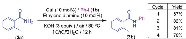
**Scheme 3** CuI-catalyzed Goldberg type C–N coupling between iodobenzene (**1b**) and 2-methylbenzamide (**2a**) under air and at 80 °C in the eutectic mixture 1ChCl/2H<sub>2</sub>O: recycling studies.
