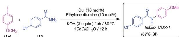
**Scheme 4** Synthesis of the biologically active aromatic secondary amide **3l** through CuI-catalyzed Goldberg type C–N coupling between 4-iodoanisole (**1e**) and 4-chlorobenzamide (**2f**), under air and at 80 °C in the eutectic mixture 1ChCl/2H<sub>2</sub>O.
