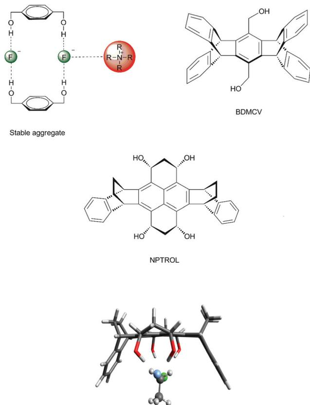
**Fig. 8** Formation of aggregates of 1,4-benzenedimethanol with fluoride ions and tetrabutylammonium counter ions. Two proposed structures (BDMCV and NPTROL) with a molecular cavity able to avoid aggregation. The bottom structure is the  $S_N2$  transition state inside the NPTROL cavity.
