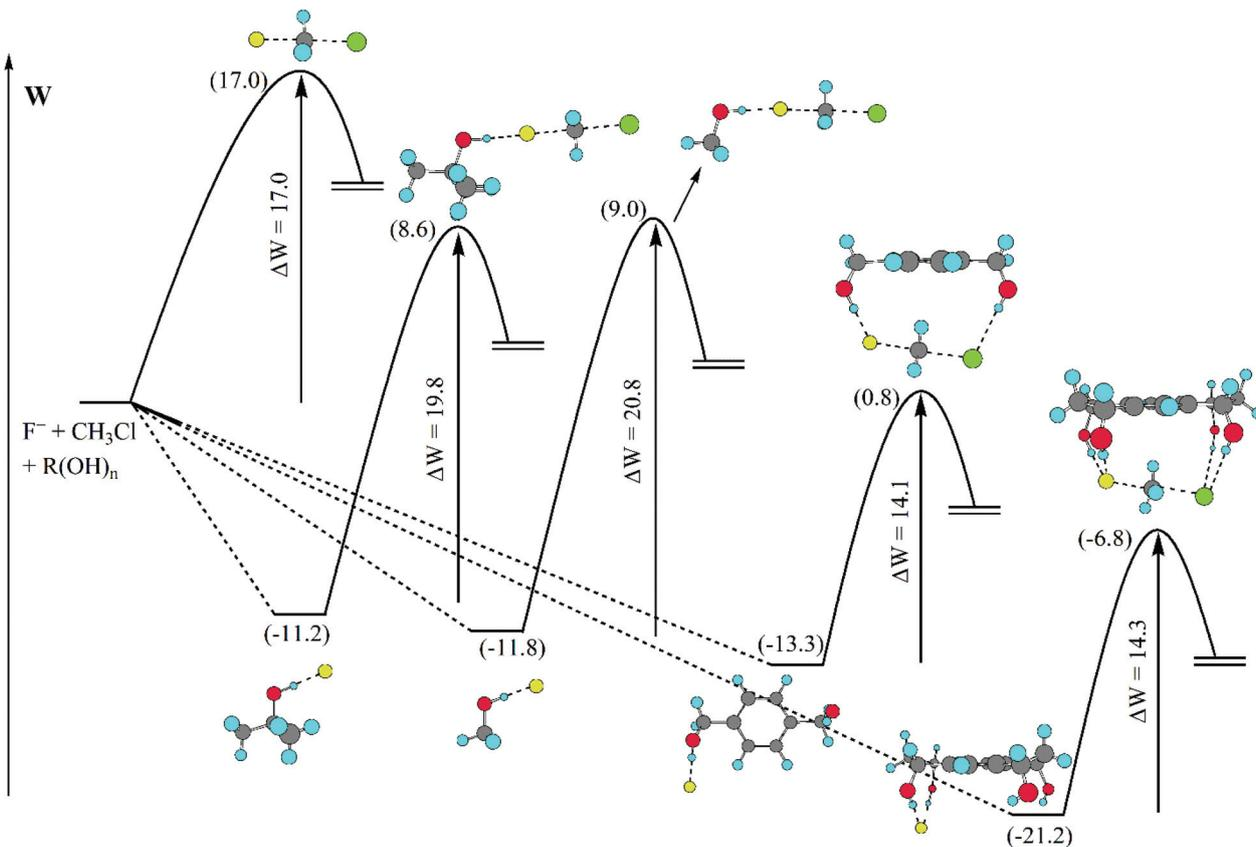
Fig. 7 Effect of different alcohols on the potential of mean force barrier for a model  $S_N2$  reaction in DMSO solvent determined by theoretical calculations. Reprinted with permission from J. R. Pliego Jr, *J. Phys. Chem. B*, 2009, **113**, 505–510. Copyright (2009) American Chemical Society.
