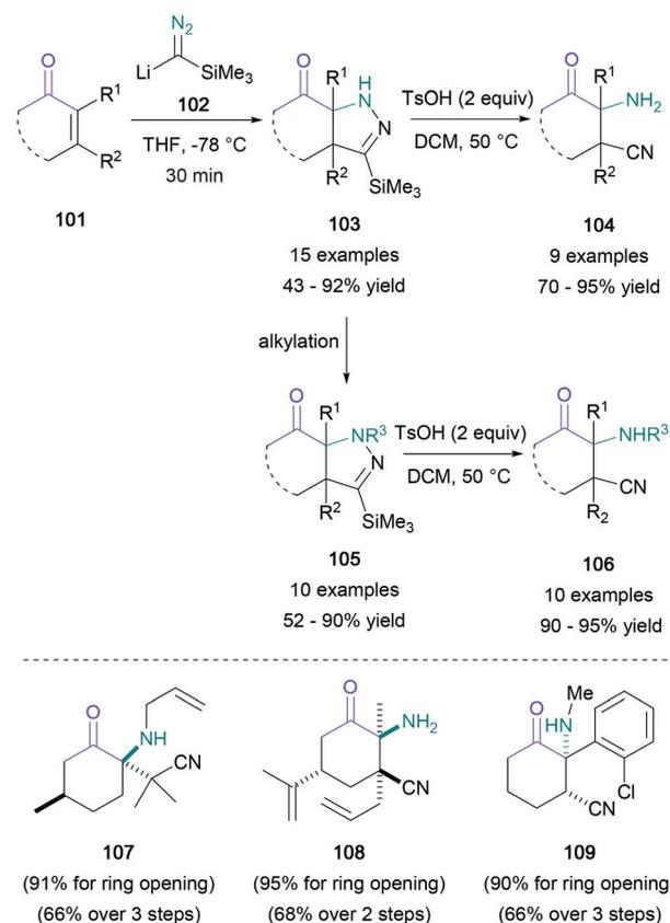
**Scheme 22** Lee's two-step synthesis of  $\alpha$ -amino ketones via pyrazolines.
