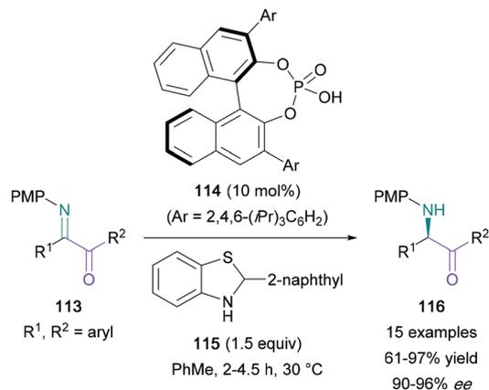
**Scheme 24** Guo's Brønsted acid-catalysed enantioselective transfer hydrogenation of imines.
