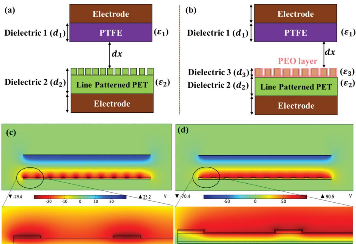
Fig. 2 (a) and (b) Schematic diagram of single and DL<sub>2</sub> TENG in the contact separation mode, (c) and (d) COMSOL Multiphysics simulation of pristine and the PEO coated LP PET TENG device.
