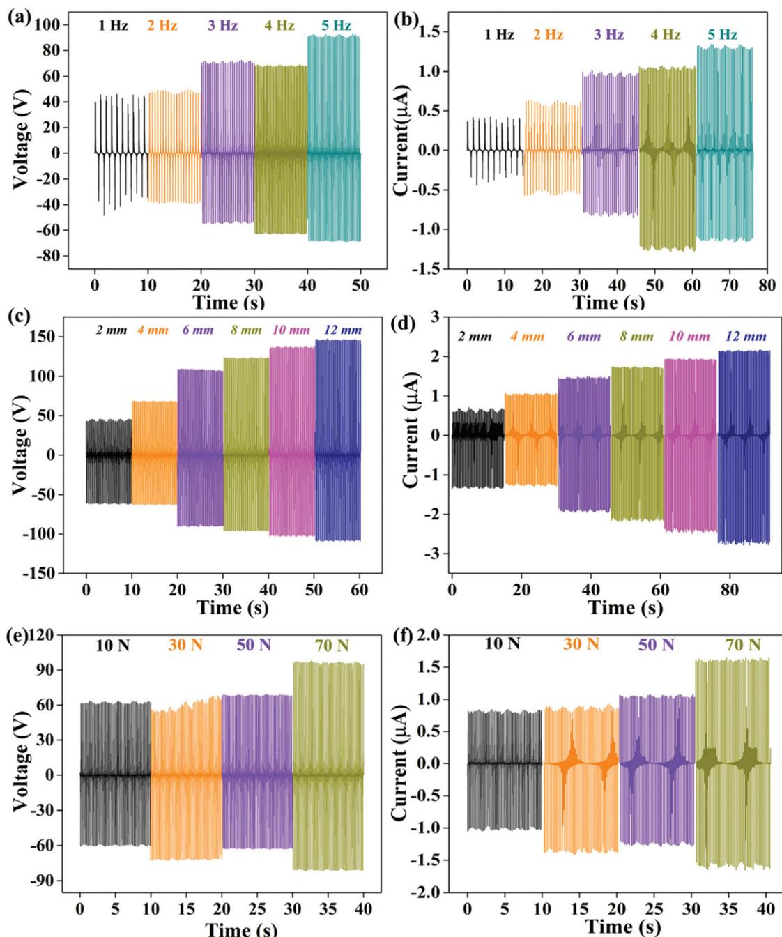
Fig. 4 (a) and (b)  $V_{oc}$  and  $I_{sc}$  of DL<sub>1</sub>/DL<sub>2</sub> TENG with various frequencies (1–5 Hz); CS distance and load were fixed at 4 mm, and 50 N, (c) and (d)  $V_{oc}$  and  $I_{sc}$  evaluation under different CS distances (2 to 12 mm) with a constant load of 50 N and frequency of 4 Hz, (e) and (f) shows the performance of  $V_{oc}$  and  $I_{sc}$  for different contact forces (10–70 N) with a constant frequency and CS distance (4 Hz and 4 mm).
