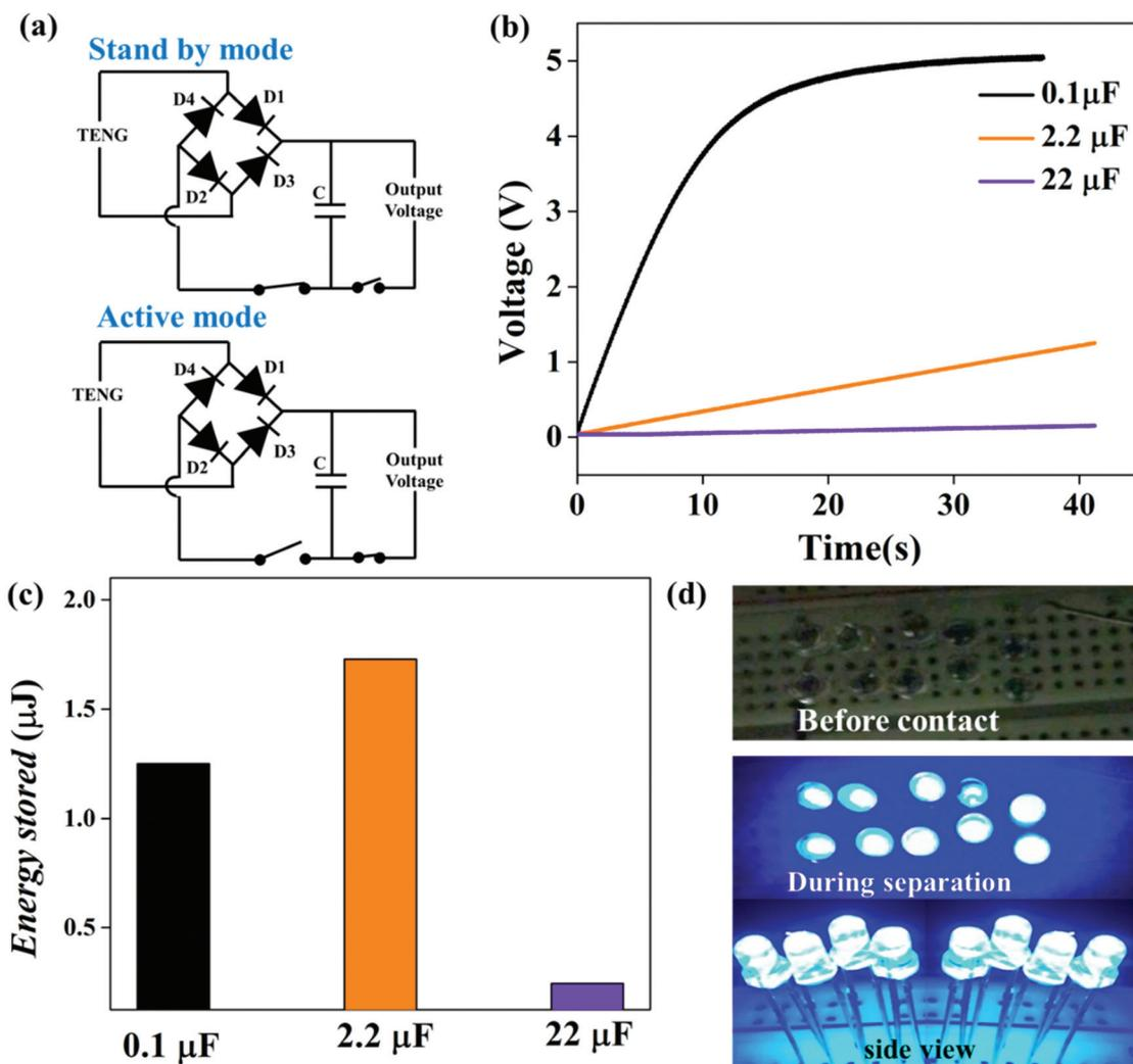
Fig. 6 Schematic diagram of the charging circuit (a) and (b) the DL<sub>2</sub> device deployed to generate the voltage stored in different capacitors, (c) the amount of energy stored in various capacitors, and (d) the digital image of ten LEDs lightened up by charged capacitor.
