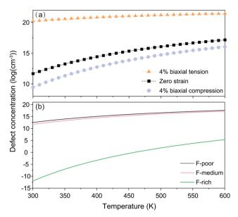
Fig. 5 (a) Concentrations of neutral  $OH_F$  defects (under different strains) as a function of temperature under F-medium conditions. (b) Concentrations of neutral  $OH_F$  defects (strain-free) as a function of temperature under three representative conditions.
