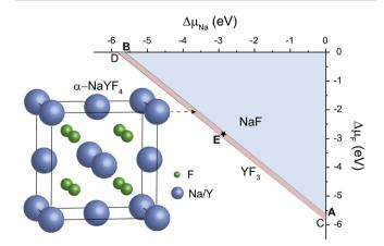
Fig. 1 Atomic illustration of cubic-phase NaYF<sub>4</sub> and the corresponding thermodynamic stability diagram as a function of the relative chemical potentials of sodium ( $\Delta \mu_{Na}$ ) and fluoride ( $\Delta \mu_{E}$ ). Points A, E, and B represent three sets of chemical potentials.
