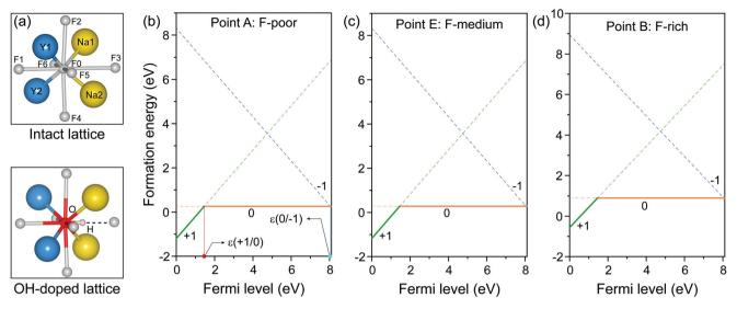
Fig. 2 (a) Optimized first coordination shell of F<sup>-</sup> (upper panel) and OH<sup>-</sup> (lower panel) ions. (b-d) Formation energies of OH<sub>F</sub> defects as a function of Fermi energy under F-poor, F-medium, and F-rich conditions (points A, E, and B in Fig. 1).  $OH_F$  denotes the substitution of  $F^-$  by  $OH^-$ , and  $\varepsilon$  is the corresponding thermodynamic transition level.
