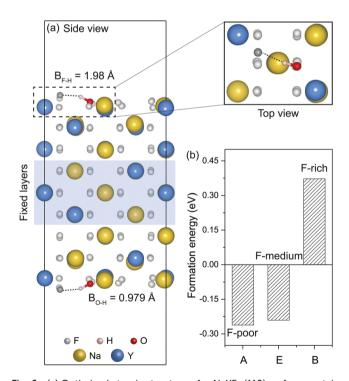
Fig. 6 (a) Optimized atomic structure of  $\alpha$ -NaYF $_4$  (110) surface containing neutral OH $_F$  defects. (b) Formation energies of the corresponding OH $_F$  defects under three representative conditions.  $B_{F-H}$  and  $B_{O-H}$  denote the length of F–H and O–H bonds, respectively.
