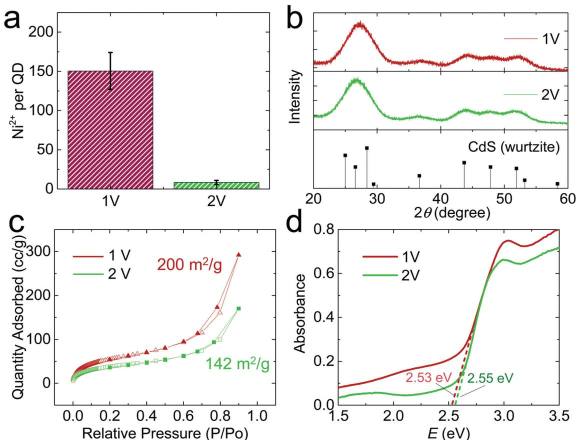
**Fig. 2** Compositional and structural characterization of QD electrogels synthesized at 1 V and 2 V. (a)  $\text{Ni}^{2+}$ /QD ratio in the gels. (b) Powder X-ray diffraction (PXRD) patterns. The stick diagram shows the PXRD pattern of hexagonal CdS (wurtzite) as a reference. (c) Nitrogen adsorption–desorption isotherms. (d) Solid-state diffuse reflectance data (converted to absorbance).
