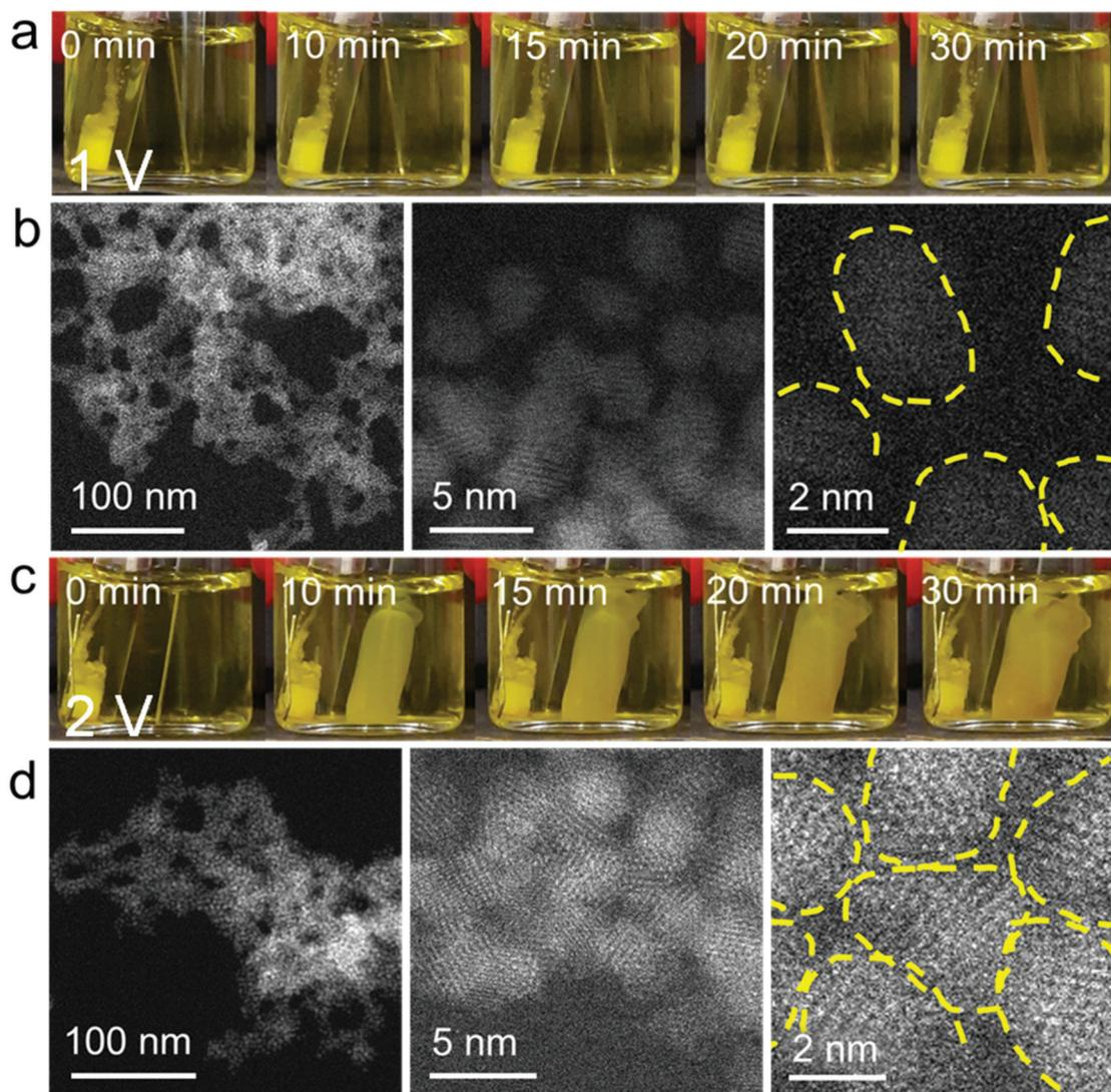
**Fig. 1** Electrodeposition of MUA-capped CdS QDs using a Ni electrode at  $E = 1$  V and 2 V Ag/AgCl/sat. KCl reference electrode. (a and b) photographs and STEM images of a QD gel grown at 1 V. (c and d) photographs and STEM images of a QD gel grown at 2 V. The yellow dashed lines in the high-magnification STEM images highlight the boundaries of individual QDs in the gel.
