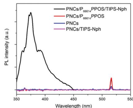
**Fig. 4** UC emission spectra of PNCs/P<sub>66614</sub>PPOS/TIPS-Nph (black), PNCs/P<sub>66614</sub>PPOS (red), PNCs (blue) and PNCs/TIPS-Nph (pink) in deaerated toluene ( $\lambda_{\text{ex}} = 515$  nm, 450 nm short-pass filter,  $I_{\text{ex}} = 80.3$  W cm<sup>-2</sup>).
