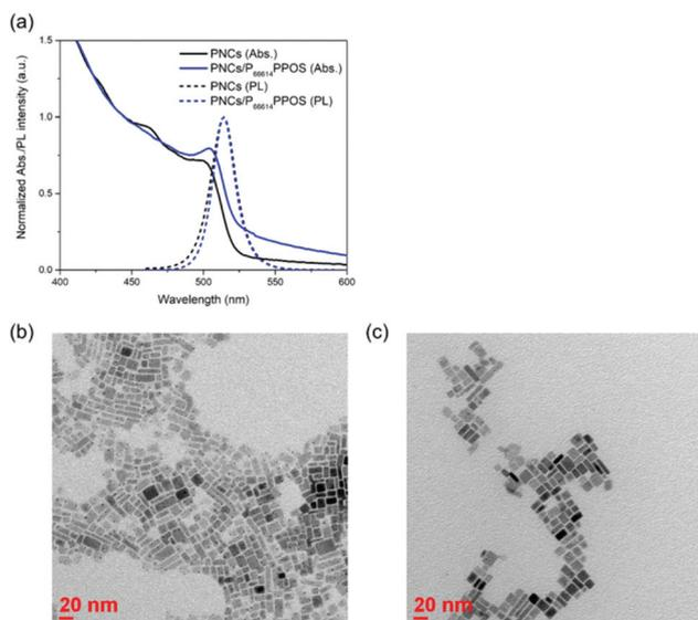
**Fig. 2** (a) Normalized absorption (solid lines, normalized at 445 nm) and photoluminescence (dashed lines,  $\lambda_{\text{ex}} = 445$  nm) spectra of purified PNCs (black) and PNCs/P<sub>66614</sub>PPOS (1 mM) (blue) in deaerated toluene. TEM images of (b) purified PNCs and (c) PNCs/P<sub>66614</sub>PPOS.
